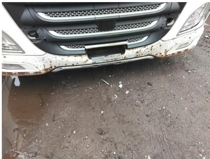
2: Bumper Front Rusted Over 5mm
