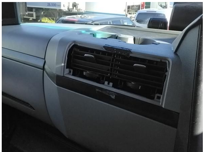
14: Air Vents nsf Damaged Replace
