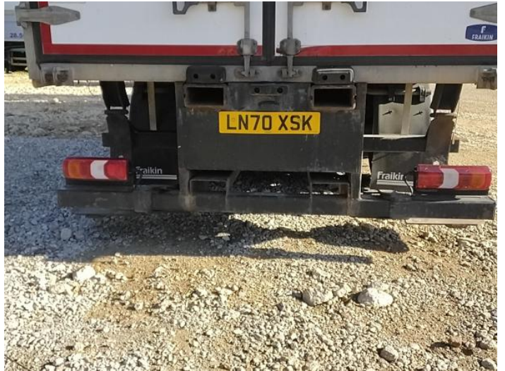
10: Bumper Rear Rusted Over 5mm
