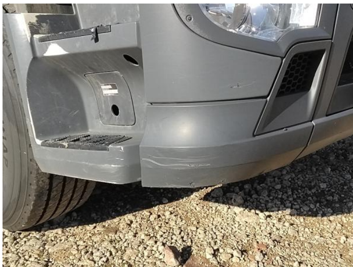
1: Bumper Front Moulding Scuffed (Unpainted) UpTo 100mm
