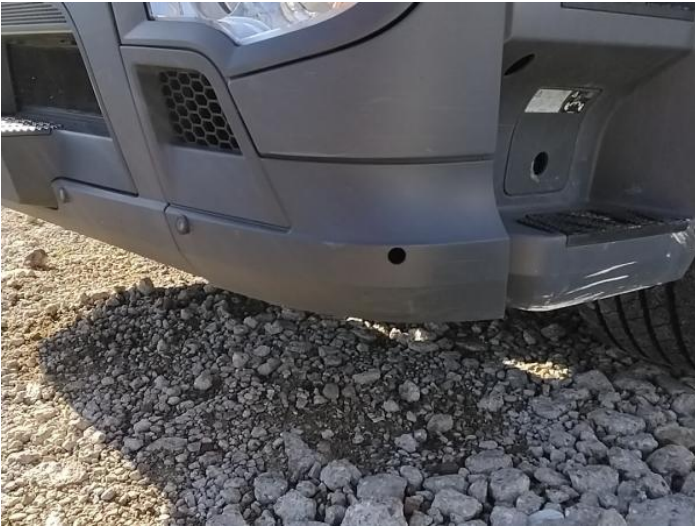
4: Bumper Front Moulding Scuffed (Unpainted) UpTo 100mm
