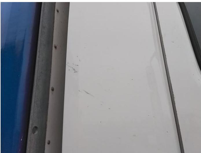
7: Qtr Panel Trim os Scuffed Over 25mm
