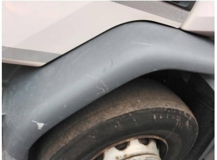
4: Wing nsf Scratched Over 25mm Thru Paint
