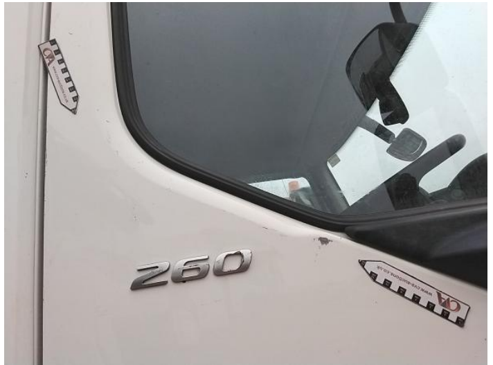
6: Door osf Scratched Over 25mm Thru Paint
