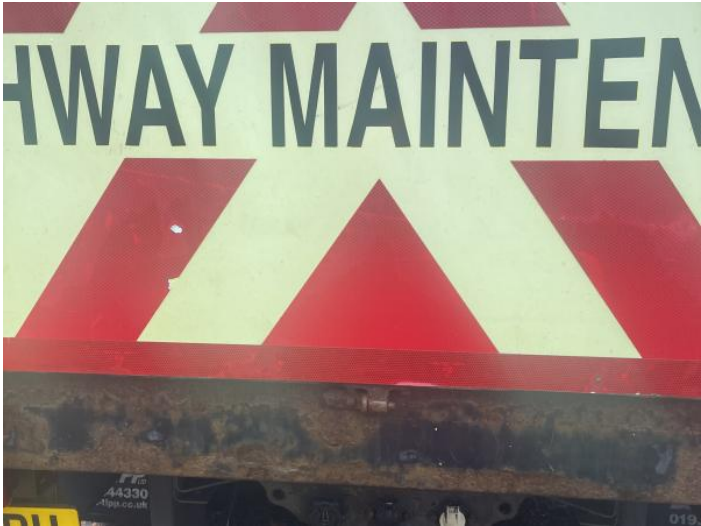
4: Tailgate Rusted Over 5mm
