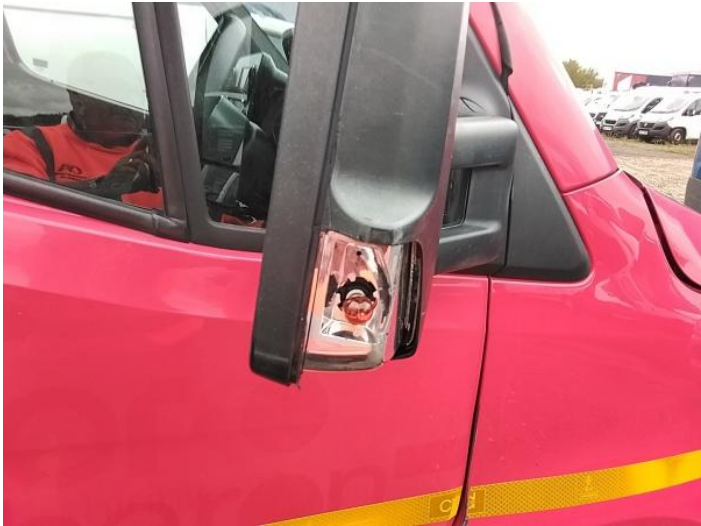
10: Door Mirror Assy osf Broken Replace
