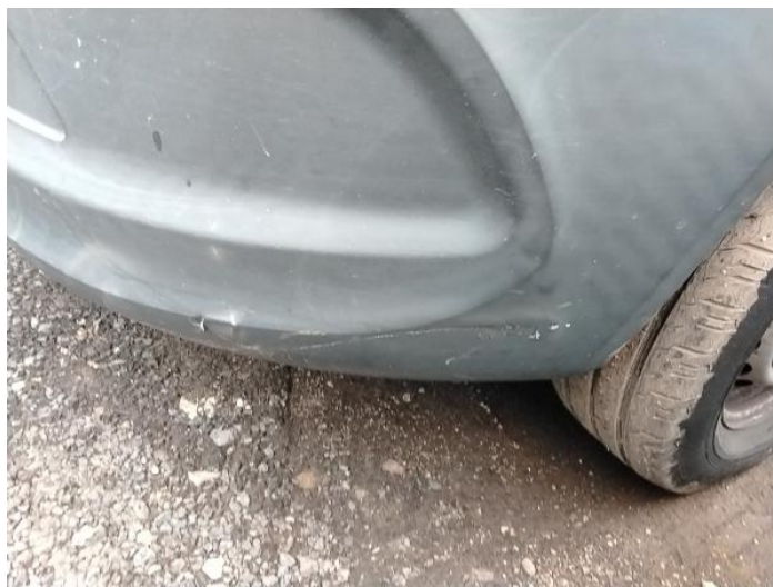
2: Bumper Front Scratched Over 100mm Thru Paint
