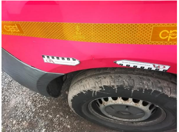
4: Wing nsf Dented With Paint Damage Over 25mm Thru Paint
