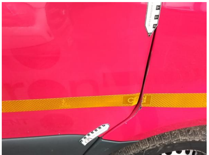
8: Door nsf Dented With Paint Damage Over 25mm Thru Paint
