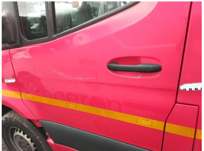
6: Door nsf Scratched Over 25mm Thru Paint
