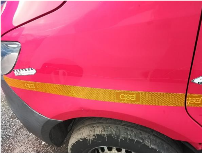
3: Wing nsf Scratched Over 25mm Thru Paint
