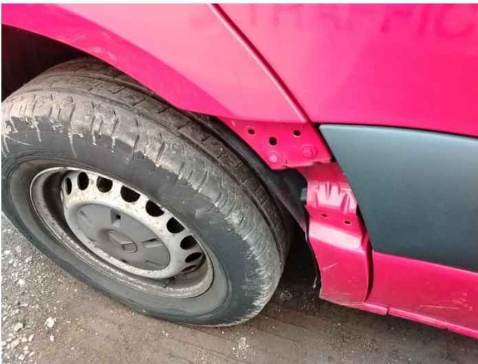
5: Door Moulding nsf Missing Replace
