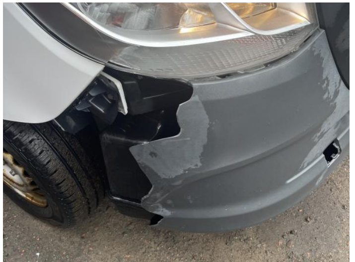
2: Bumper Front Moulding Broken Replace
