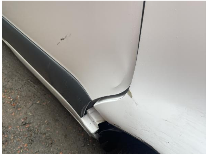
4: Door osf Dented Over 30mm
