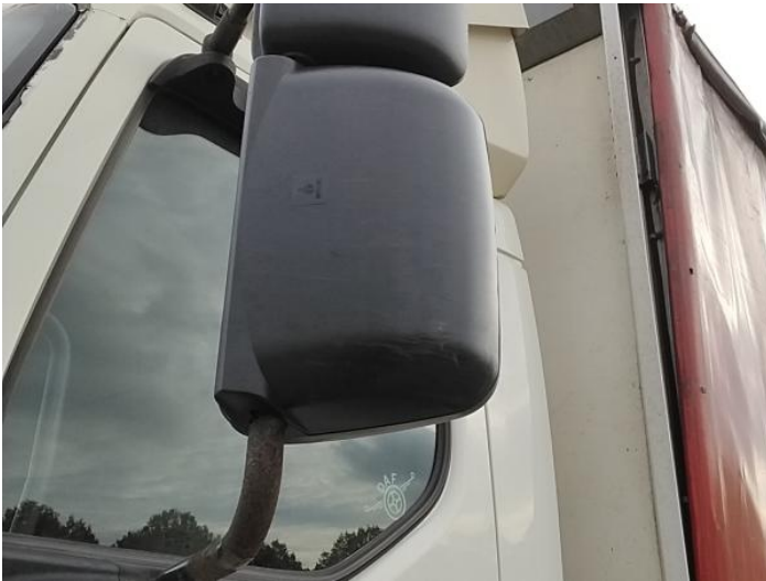
11: Door Mirror Assy nsf Scuffed (Unpainted) UpTo 100mm
