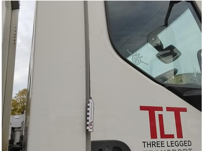
16: Door osf Chipped Edge Chip
