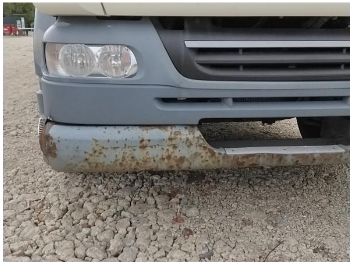
4: Bumper Front Moulding Broken Replace
