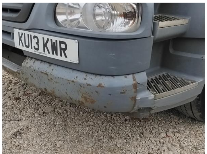
8: Bumper Front Moulding Scuffed (Unpainted) UpTo 100mm
