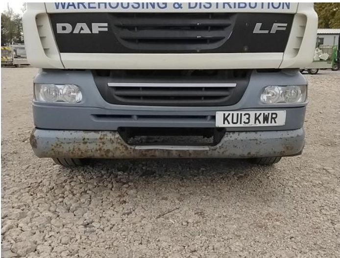
3: Bumper Front Rusted Over 5mm
