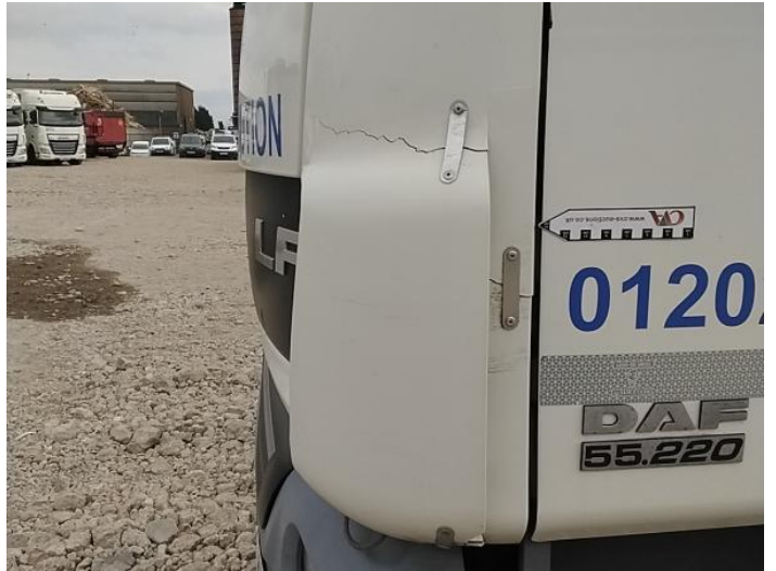
10: Wing nsf Cracked Replace
