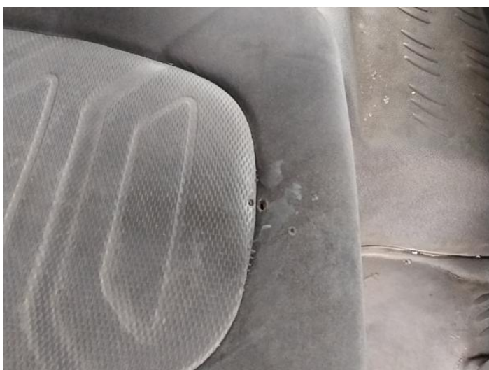
23: Seat Base Cover osf Burn Over 3mm
