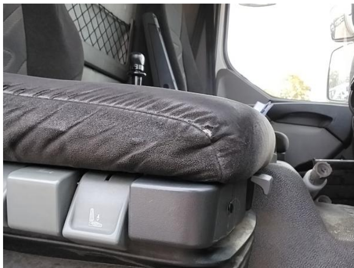
22: Seat Base Cover osf Holed Over 3mm
