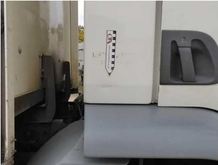
15: B Post os Dented With Paint Damage
