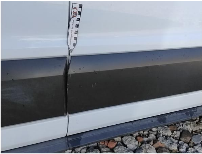
5: Door Moulding osf Scuffed (Unpainted) UpTo 100mm
