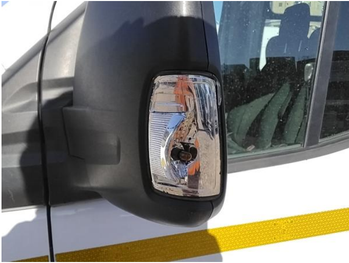
4: Flasher Side Repeater ns Broken Replace
