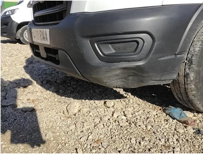
3: Bumper Front Dented Over 30mm
