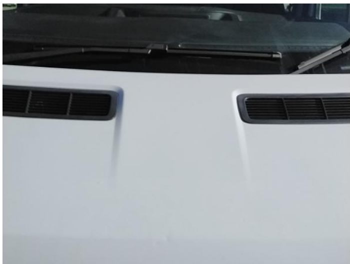
1: Bonnet Dented 2 Or Less UpTo 10mm
