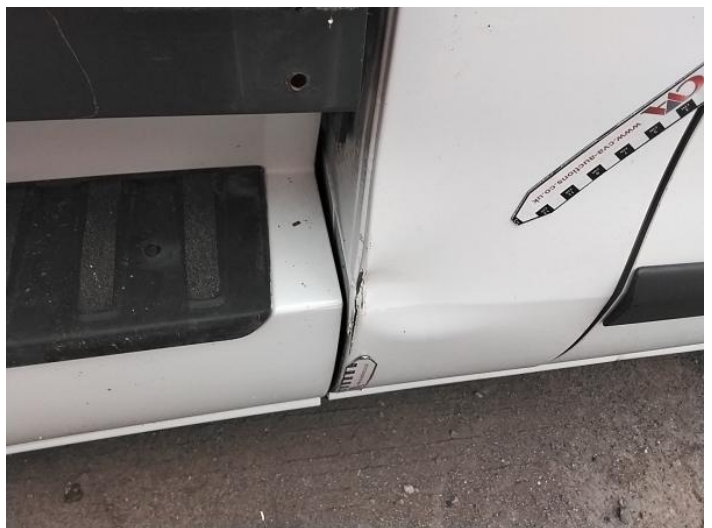
8: B Post os Dented With Paint Damage
