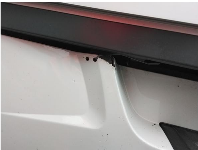
7: Qtr Panel osr Cracked Replace
