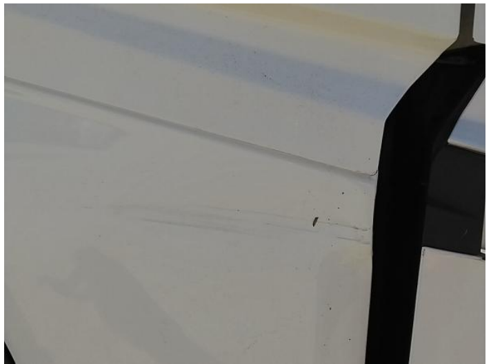
12: Door osf Dented With Paint Damage
