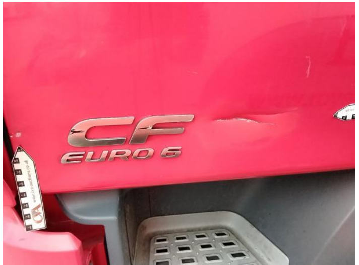
6: Door nsf Dented With Paint Damage
