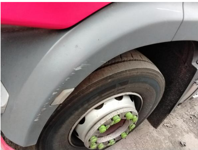
7: Wing nsf Scratched Over 25mm Thru Paint
