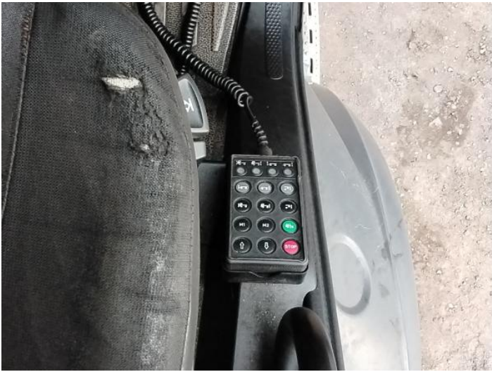
11: Seat Base Cover osf Torn Over 3mm
