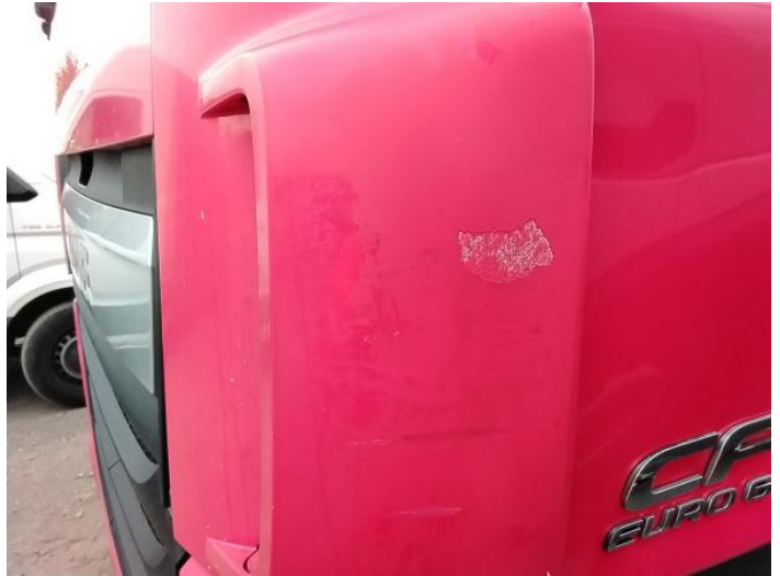
4: Panel Front Poor Previous Repair Poor Colour
