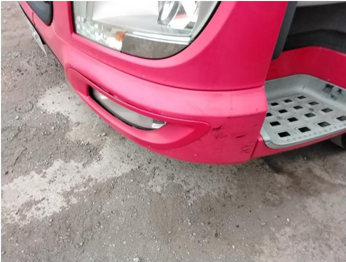
3: Bumper Front Dented With Paint Damage
