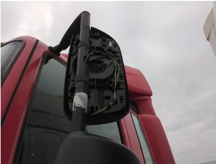
5: Door Mirror Assy nsf Broken Replace
