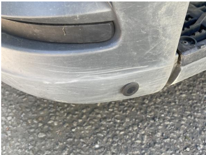
3: Bumper Front Moulding Scuffed (Unpainted) Over 100mm
