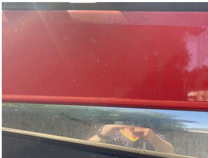
2: Bonnet Chipped Multiple Chips
