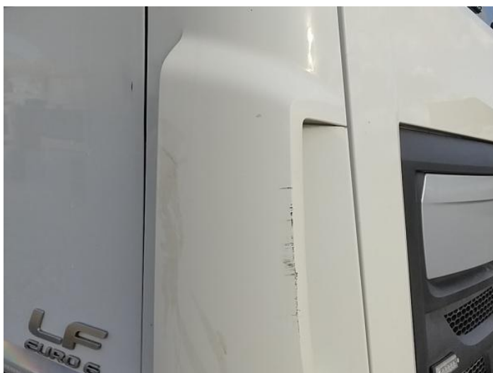
1: Wing osf Scratched Over 25mm Thru Paint
