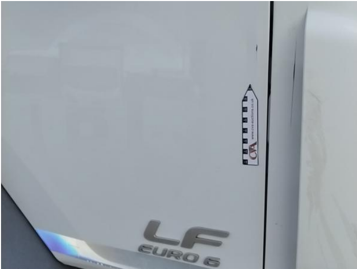
15: Door osf Scratched UpTo 25mm Thru Paint
