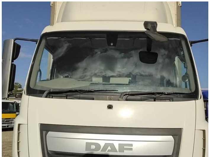
6: Screen Front Chipped Over 10mm
