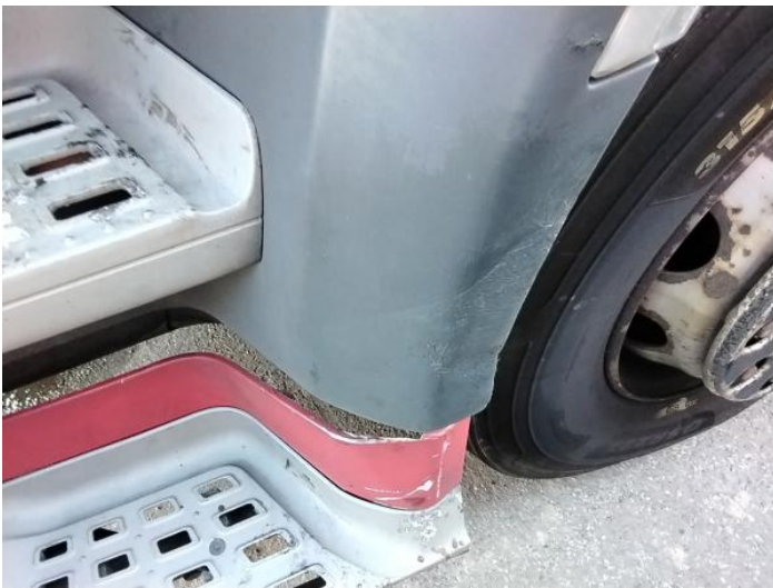
5: Wing nsf Poor Previous Repair Rippled UpTo 30%
