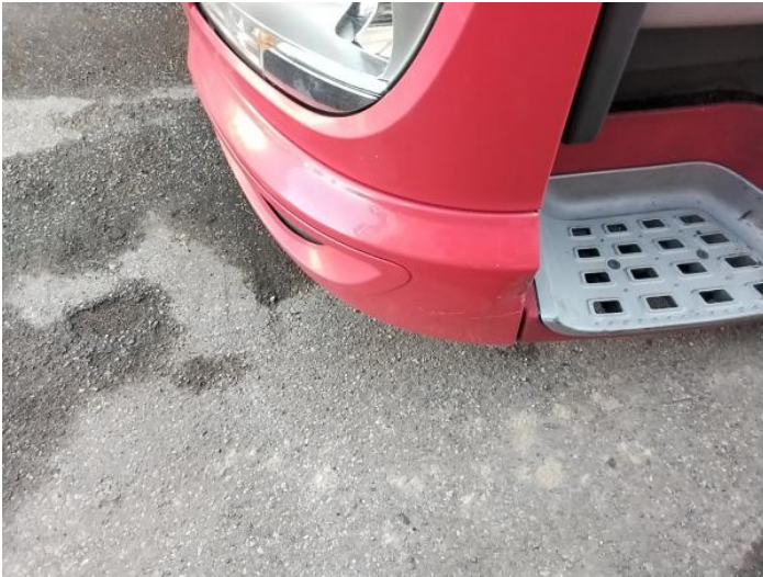
3: Bumper Front Dented With Paint Damage
