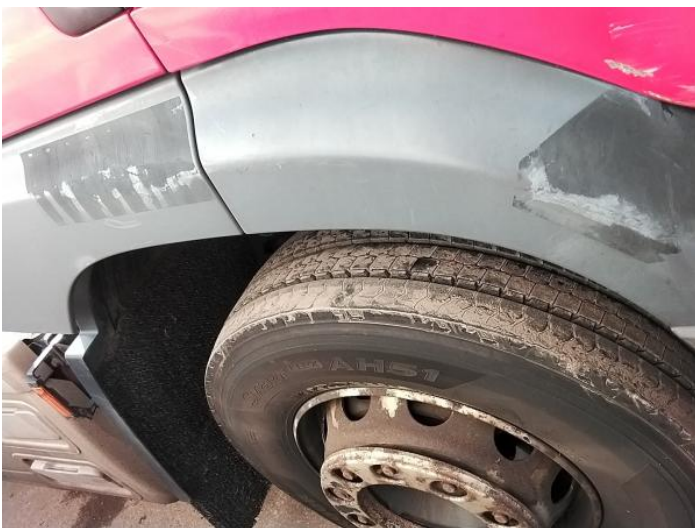
7: Wing osf Poor Previous Repair Rippled UpTo 30%
