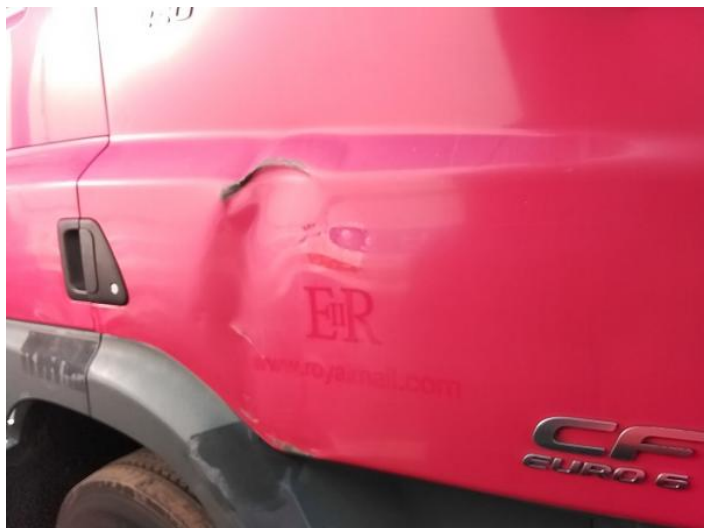
8: Door osf Dented Over 30% Of Panel
