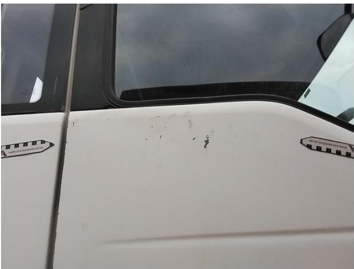
7: Door osf Dented With Paint Damage
