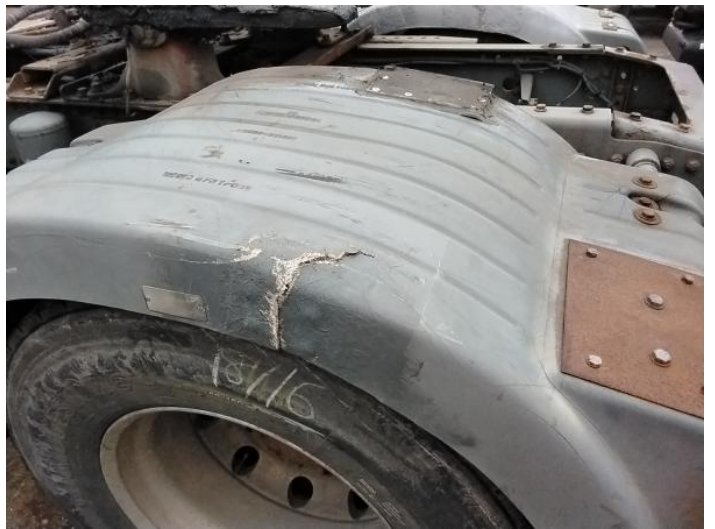
6: Qtr Panel Moulding ns Broken Replace
