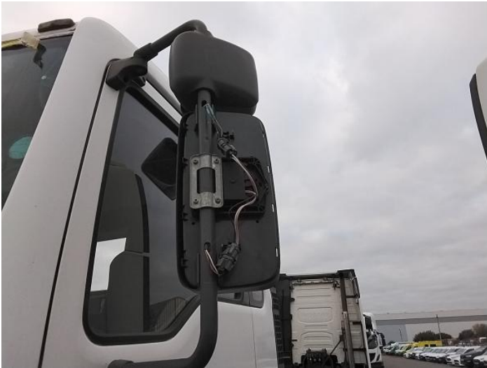
3: Door Mirror Assy nsf Broken Replace
