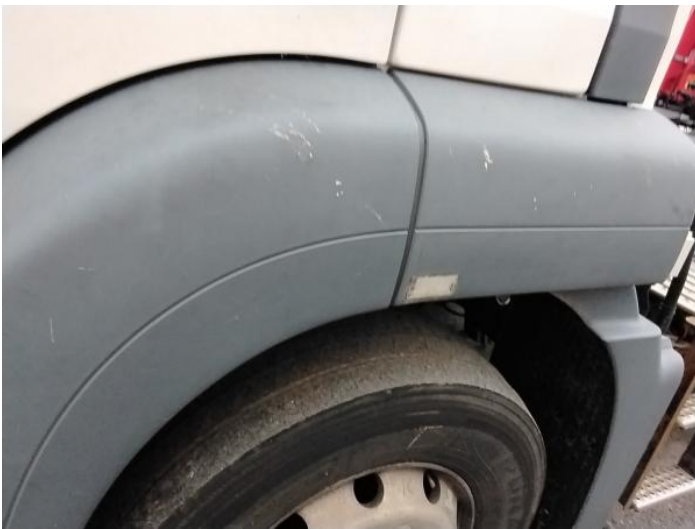
5: Wing nsf Scratched Over 25mm Thru Paint
