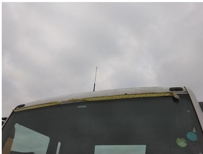
2: Aperture Seal nsf Broken Replace
