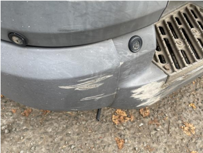
3: Bumper Front Moulding Scuffed (Unpainted) Over 100mm
