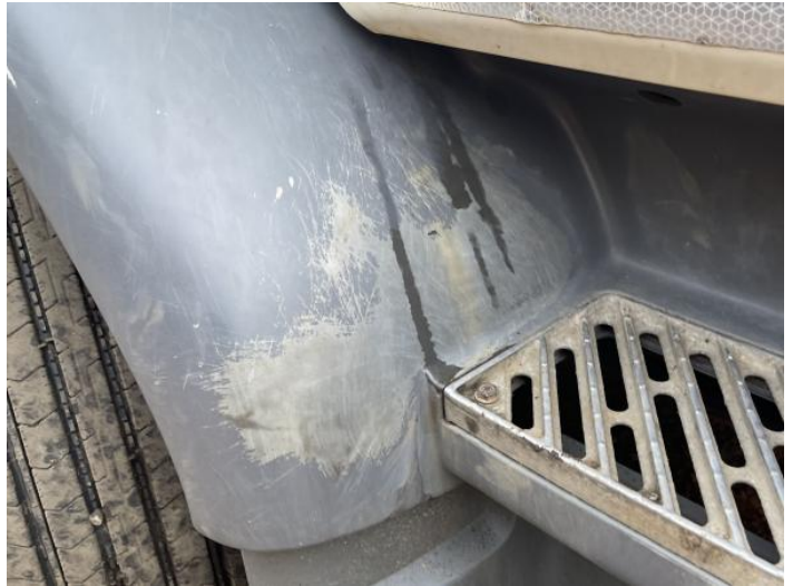
4: Door Moulding osf Scuffed (Unpainted) Over 100mm
