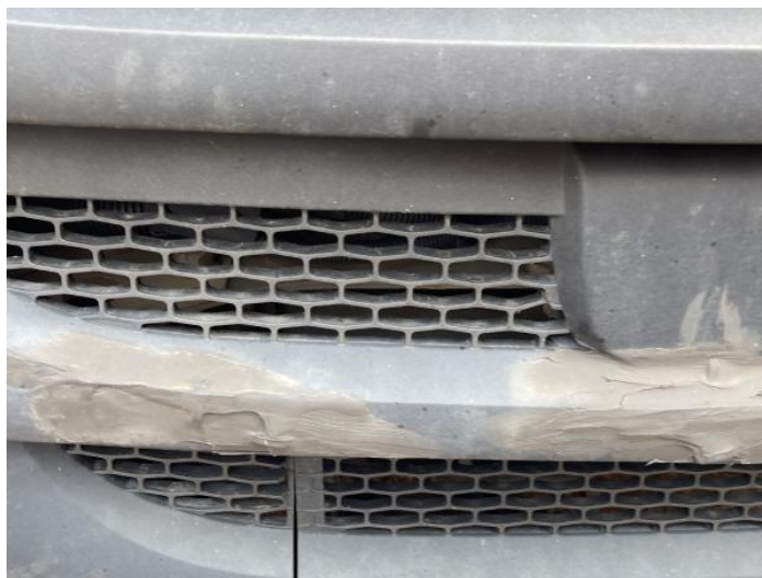
2: Bumper Front Grill Broken Replace
