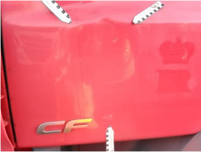
3: Door nsf Dented With Paint Damage
