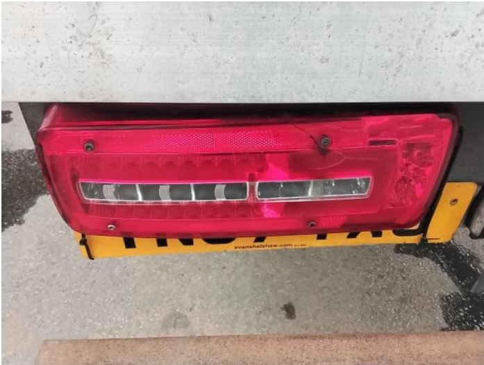
9: Lamp nsr Broken Replace
