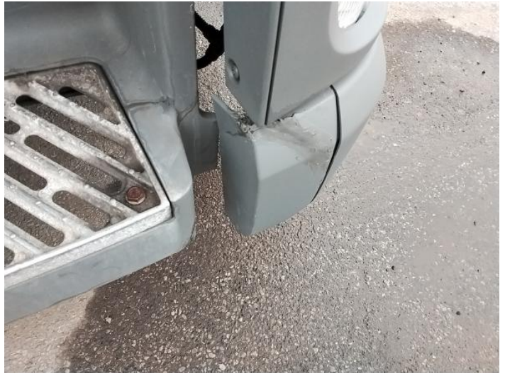
4: Bumper Front Moulding Broken Replace
