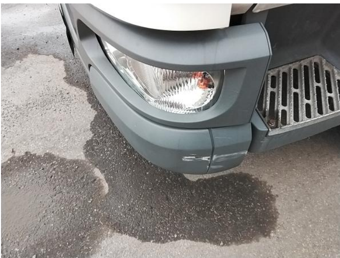
7: Bumper Front Scratched Over 100mm Thru Paint
