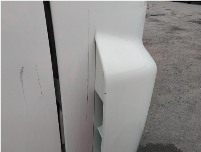
3: Panel Front Scratched Over 25mm Thru Paint
