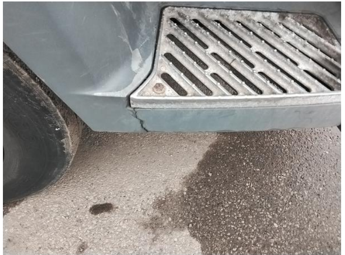
6: Bumper Front Moulding Broken Replace
