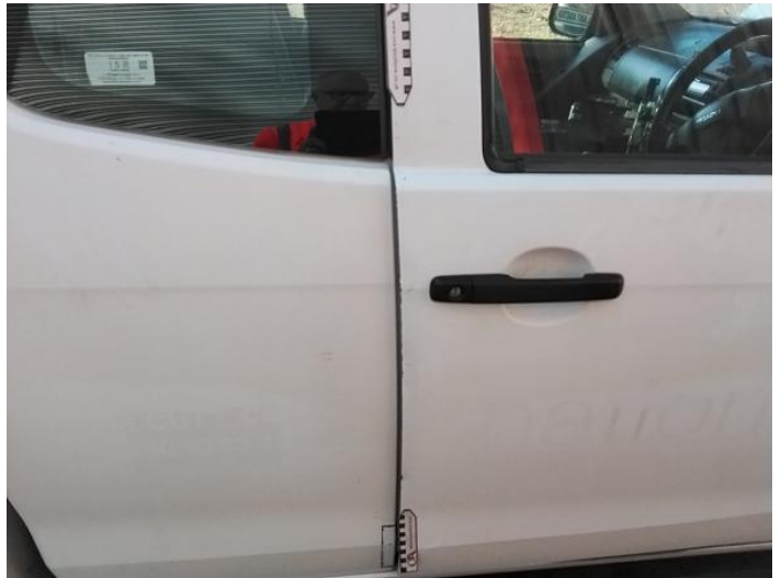
12: Door osf Dented With Paint Damage
