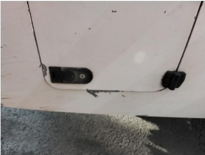
11: Qtr Panel osr Dented Over 30mm
