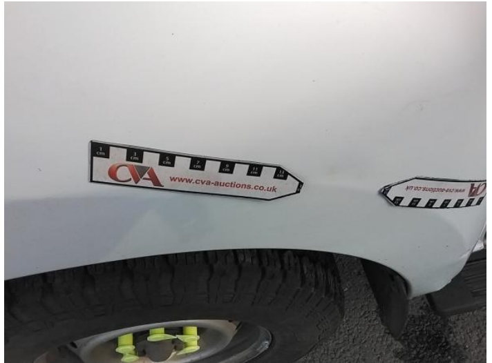
4: Wing nsf Dented Over 30mm
