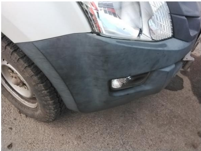
15: Bumper Front Scratched Over 100mm Thru Paint
