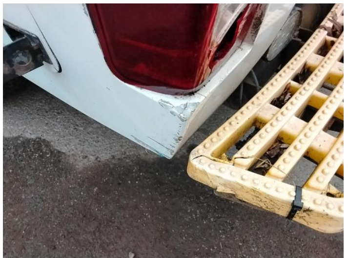
8: Qtr Panel nsr Cracked Replace
