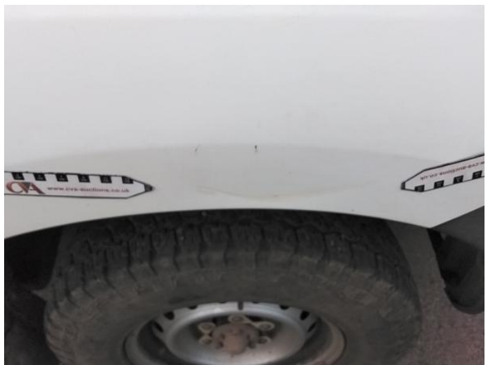
14: Wing osf Dented With Paint Damage
