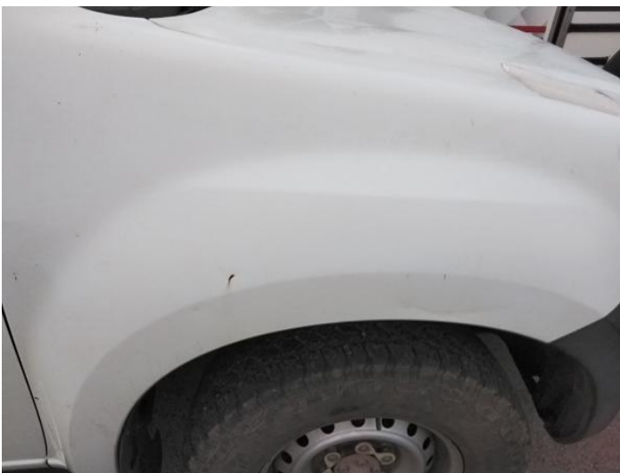
13: Wing osf Chipped Multiple Chips
