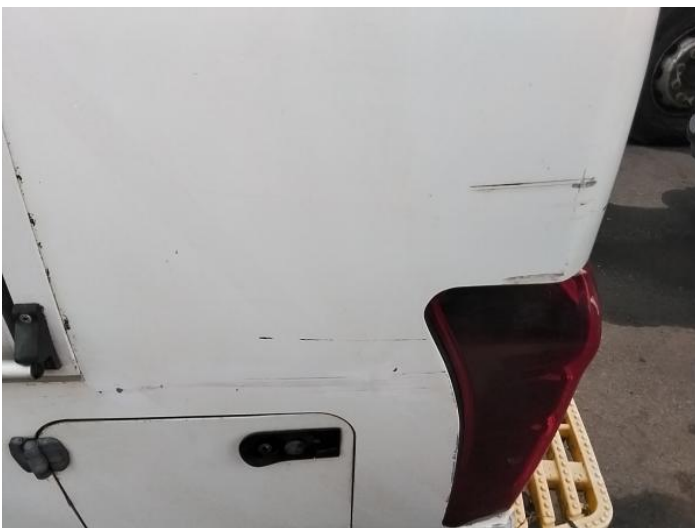
7: Qtr Panel nsr Dented With Paint Damage
