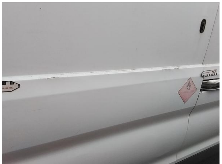
14: Qtr Panel nsr Dented With Paint Damage
