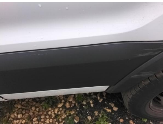
25: Qtr Panel Moulding ns Scuffed (Unpainted) Over 100mm
