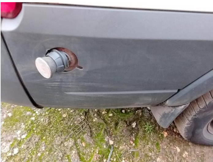
37: Qtr Panel Moulding os Scuffed (Unpainted) Over 100mm
