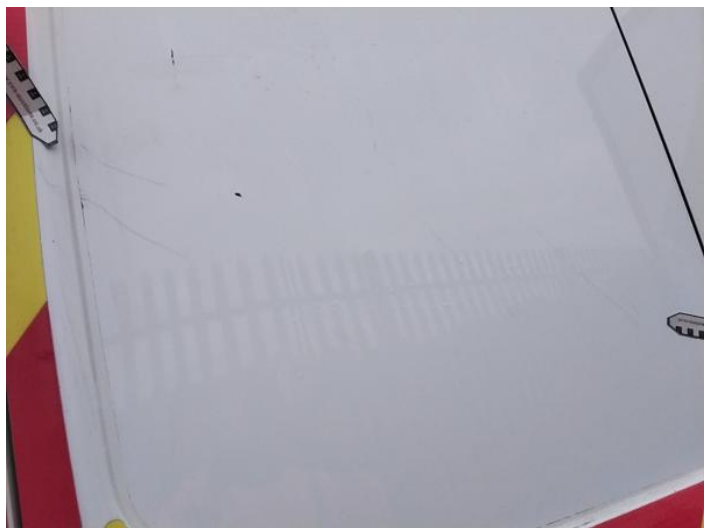
32: Door nsr Scratched Over 25mm Thru Paint
