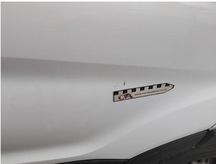
41: Door osf Scratched Over 25mm Thru Paint
