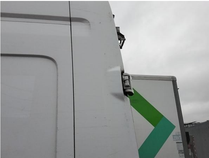
23: C Post ns Scratched Over 25mm Thru Paint
