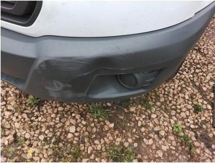
3: Bumper Front Dented With Paint Damage
