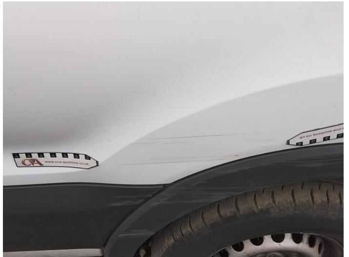
24: Qtr Panel nsr Dented With Paint Damage
