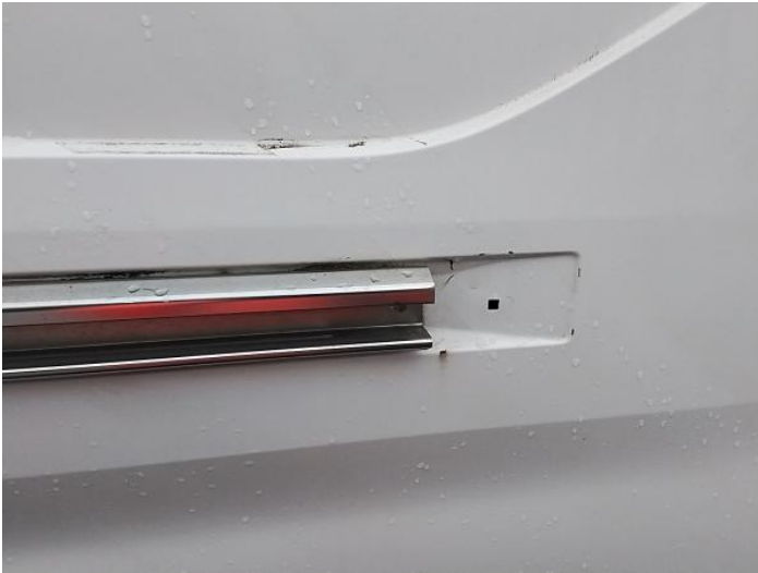
27: Qtr Panel Trim ns Missing Replace
