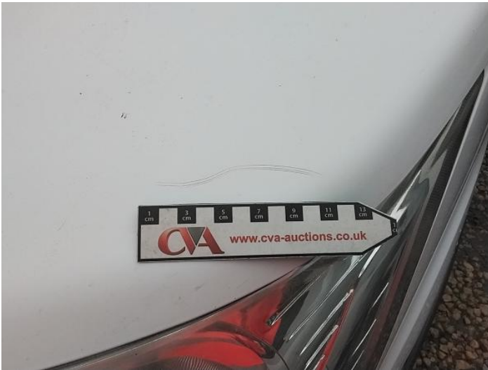
5: Bonnet Scratched Over 25mm Thru Paint
