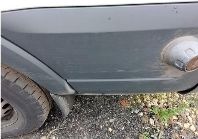
29: Qtr Panel Moulding ns Scuffed (Unpainted) Over 100mm
