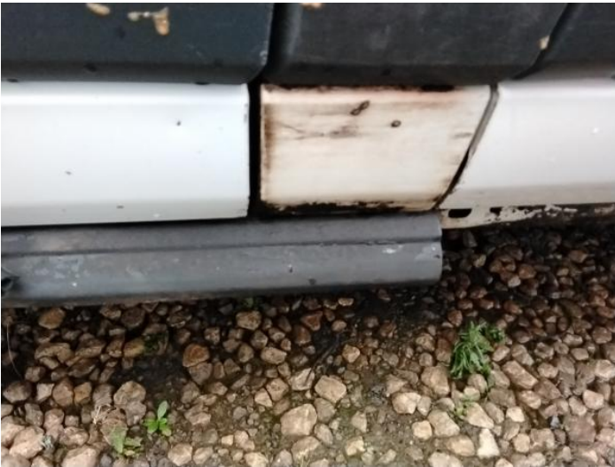
11: B Post ns Dented With Paint Damage
