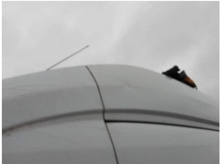
12: Roof Dented Over 30mm
