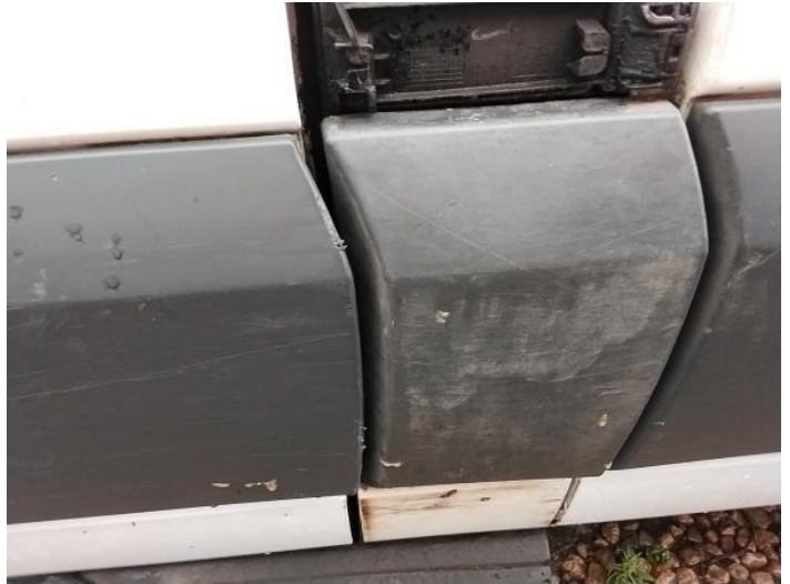
10: Door Moulding nsf Scuffed (Unpainted) UpTo 100mm
