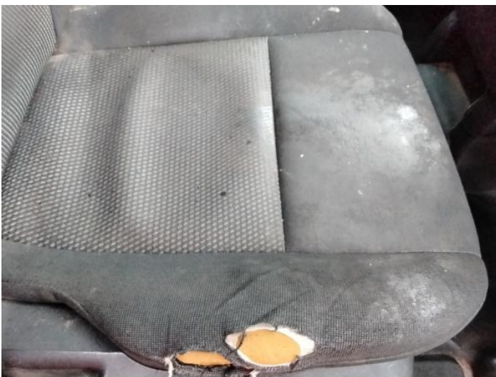
43: Seat Base Cover osf Torn Over 3mm
