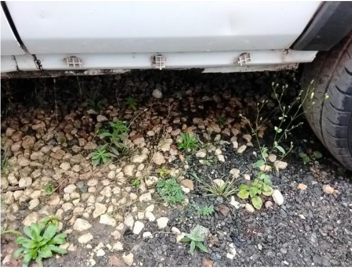
21: Qtr Panel Moulding ns Missing Replace
