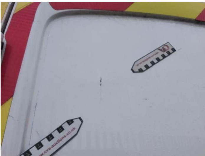
31: Door nsr Dented With Paint Damage
