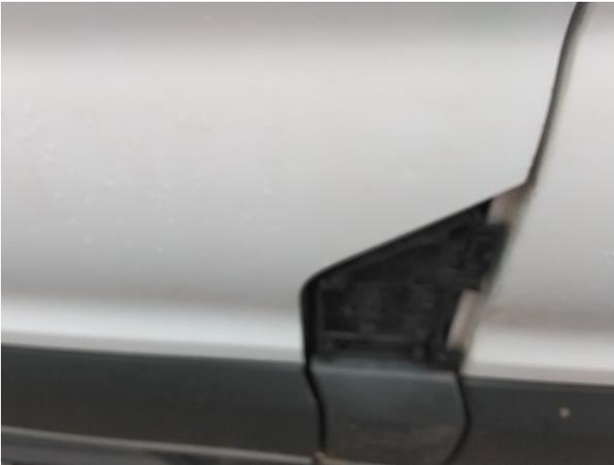
9: Fuel Flap Missing Replace
