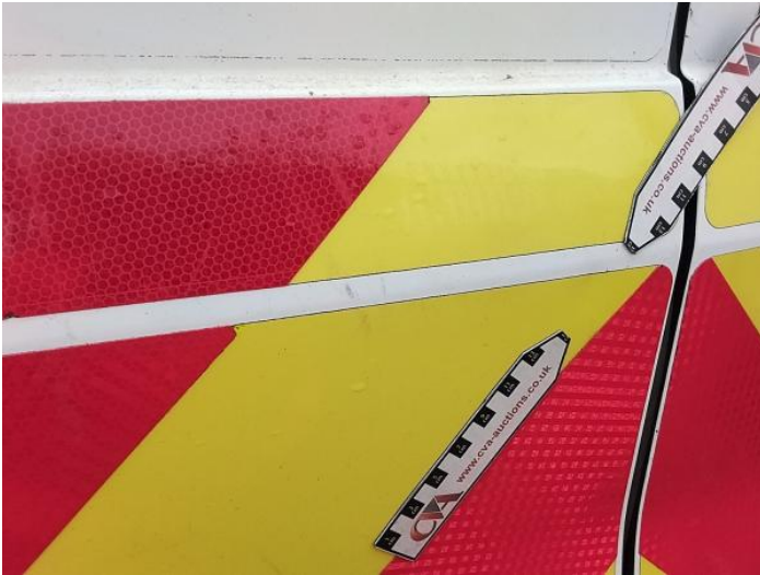
33: Door nsr Dented Over 30mm
