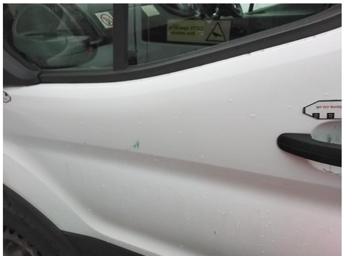
8: Door nsf Scratched Over 25mm Thru Paint
