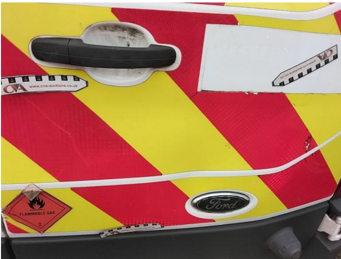
35: Door osr Dented Over 30mm
