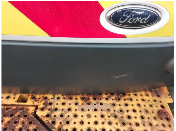
36: Door Moulding osr Scuffed (Unpainted) Over 100mm
