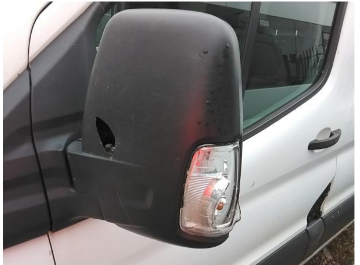
6: Door Mirror Assy nsf Broken Replace
