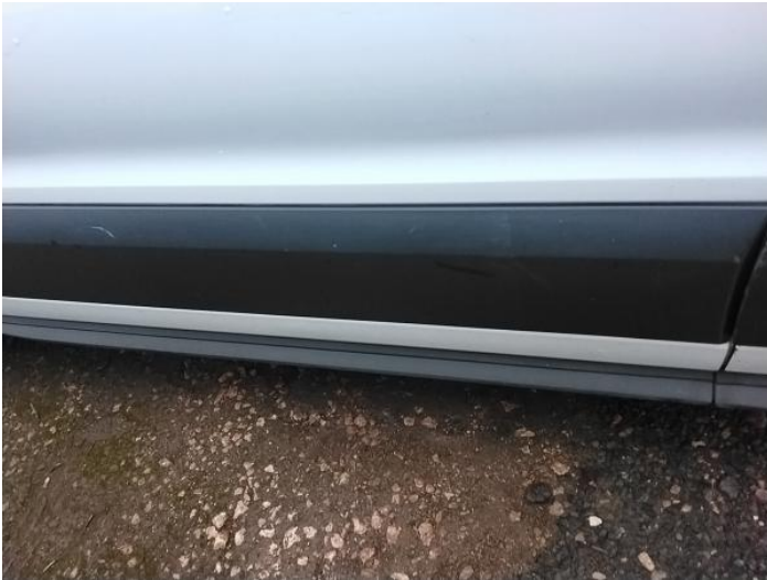
39: Qtr Panel Moulding os Scuffed (Unpainted) Over 100mm
