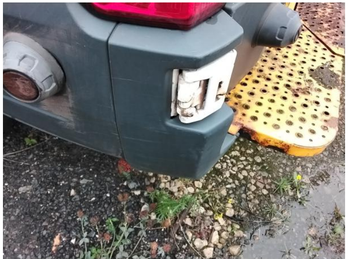
30: Bumper Rear Moulding Scuffed (Unpainted) Over 100mm
