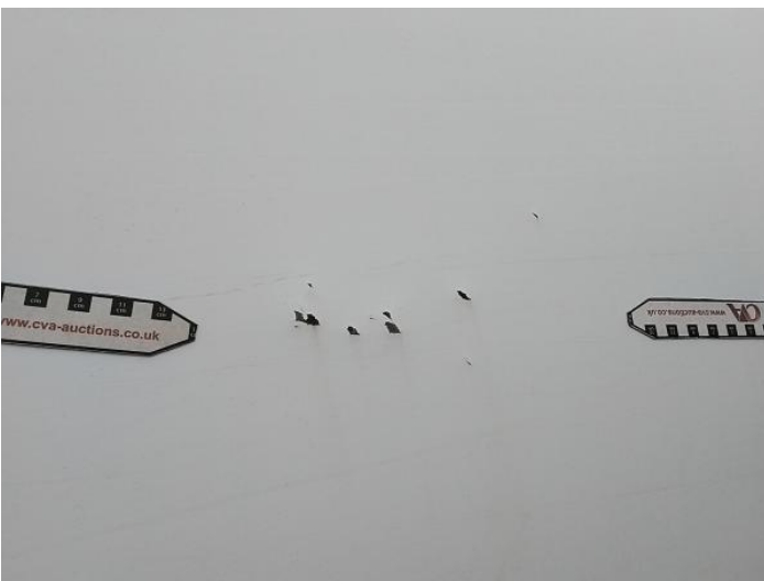
13: Qtr Panel nsr Dented With Paint Damage
