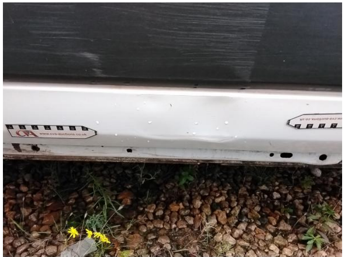
18: Qtr Panel nsr Dented With Paint Damage
