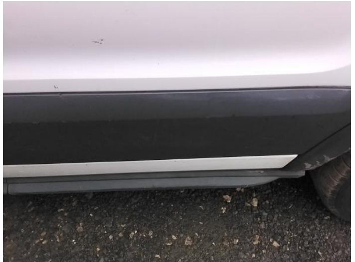
40: Door Moulding osf Scuffed (Unpainted) Over 100mm
