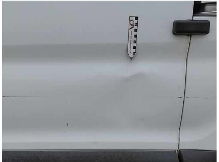
10: Door nsr Dented Over 30mm
