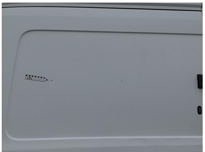
8: Door nsr Chipped Over 5mm
