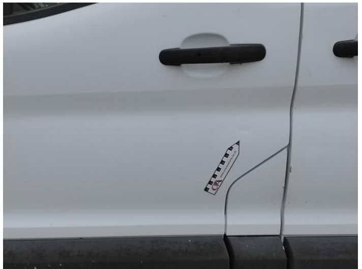
6: Door nsf Dented Over 2 UpTo 10mm
