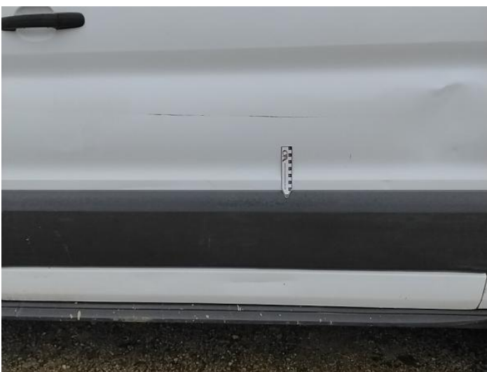
13: Door Moulding nsr Scuffed (Unpainted) Over 100mm
