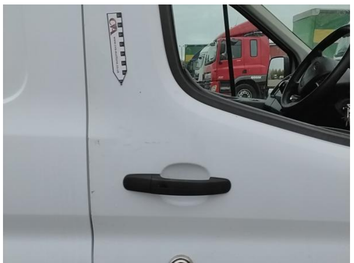
20: Door osf Scratched UpTo 25mm Not Thru Paint
