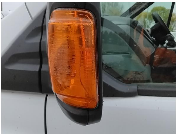
7: Flasher Side Repeater ns Broken Replace
