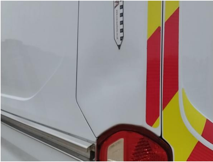
15: Qtr Panel nsr Dented Over 30mm
