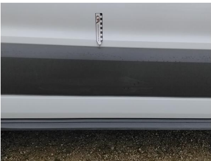
19: Qtr Panel Moulding os Scuffed (Unpainted) UpTo 100mm
