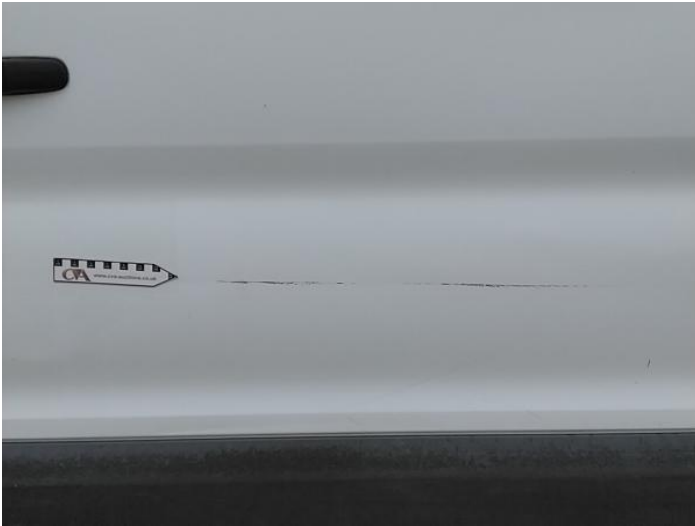
9: Door nsr Scratched Over 25mm Thru Paint
