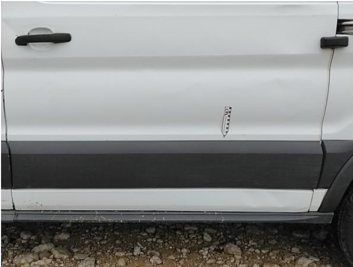
15: Door Moulding nsr Scuffed (Unpainted) UpTo 100mm
