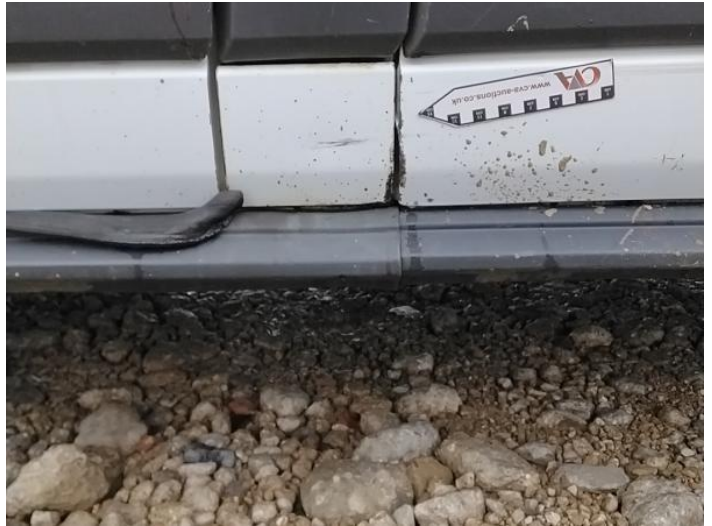
10: Door nsr Scratched UpTo 25mm Thru Paint
