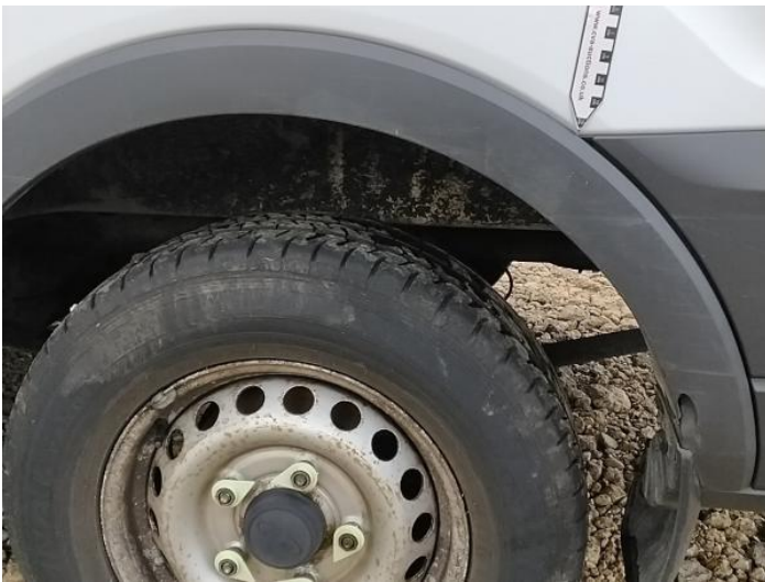
17: Qtr Panel Arch Extension ns Broken Replace
