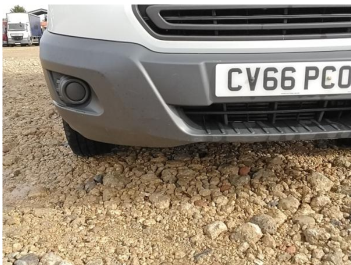
1: Bumper Front Moulding Scuffed (Unpainted) UpTo 100mm
