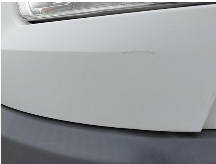
7: Panel Front Scratched UpTo 25mm Thru Paint
