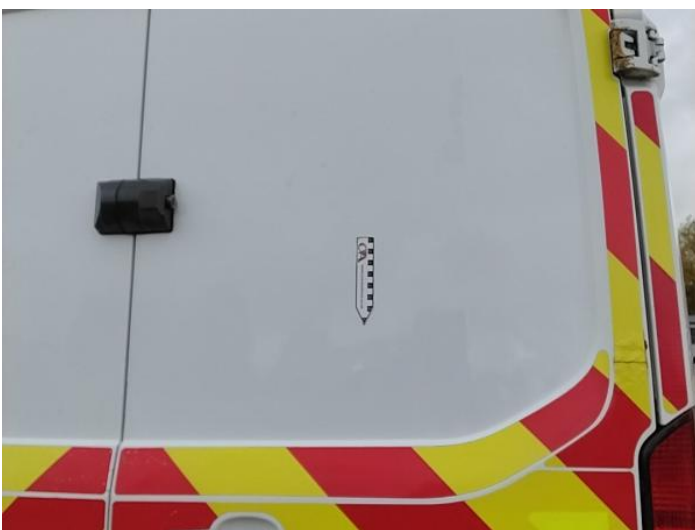
19: Door osr Dented Between 10mm + 30mm
