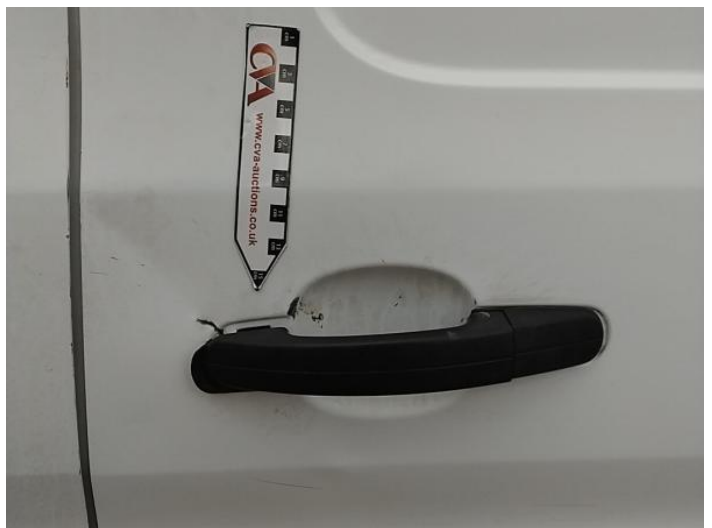
8: Handle Outer nsr Broken Replace
