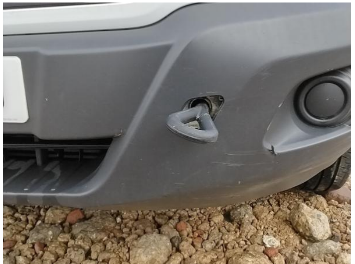
4: Front TowEye Cvr Missing Replace
