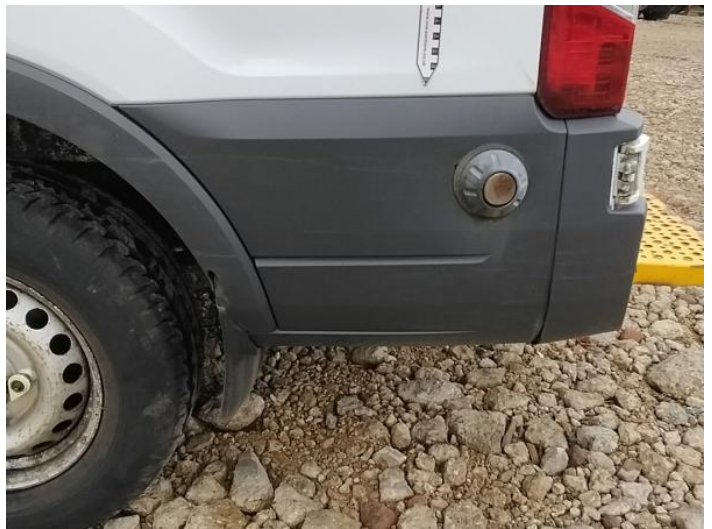
18: Qtr Panel Trim ns Scuffed Over 25mm
