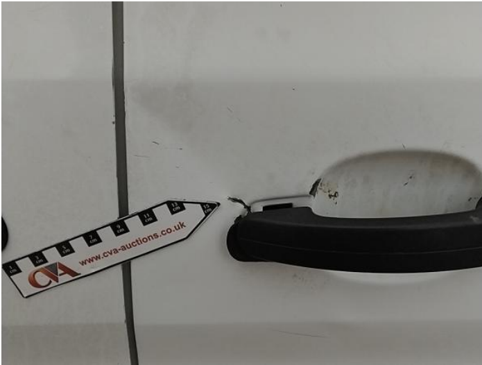
9: Door nsr Hole Over 10mm
