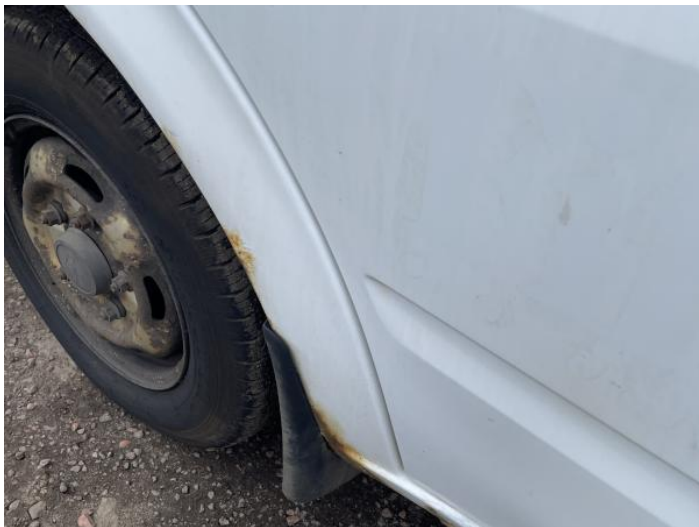
9: Door nsf Rusted Over 5mm
