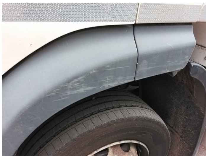
2: Wings Scratched Over 25mm Thru Paint
