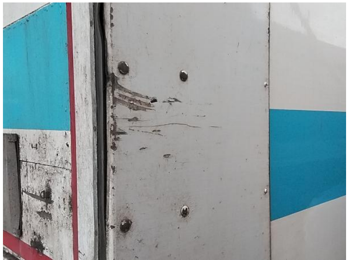
6: Qtr Panel Trim os Scuffed Over 25mm
