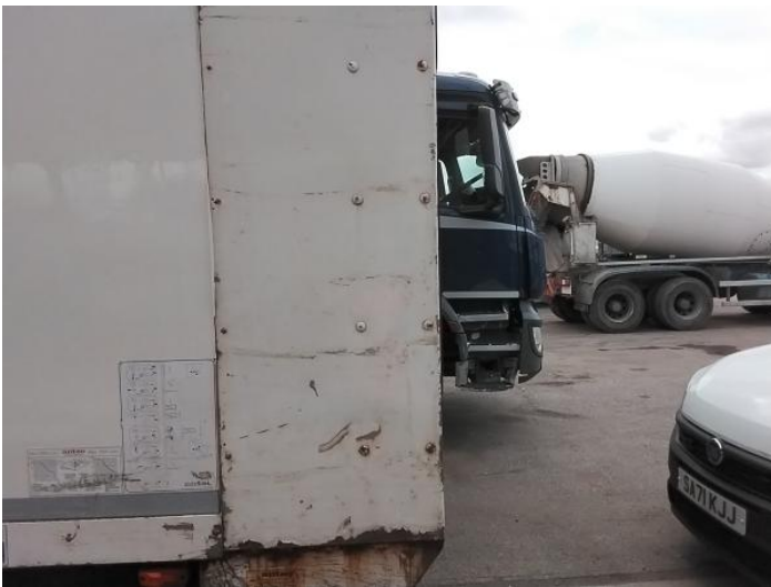
5: Qtr Panel Trim ns Scuffed Over 25mm
