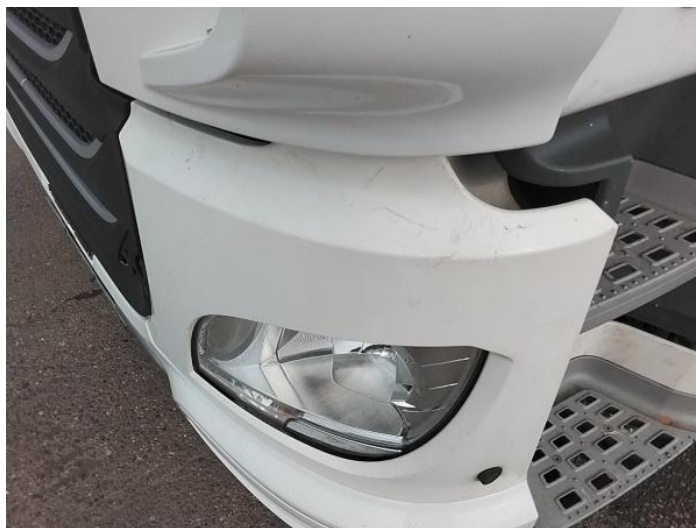
2: Panel Front Scratched Over 25mm Thru Paint
