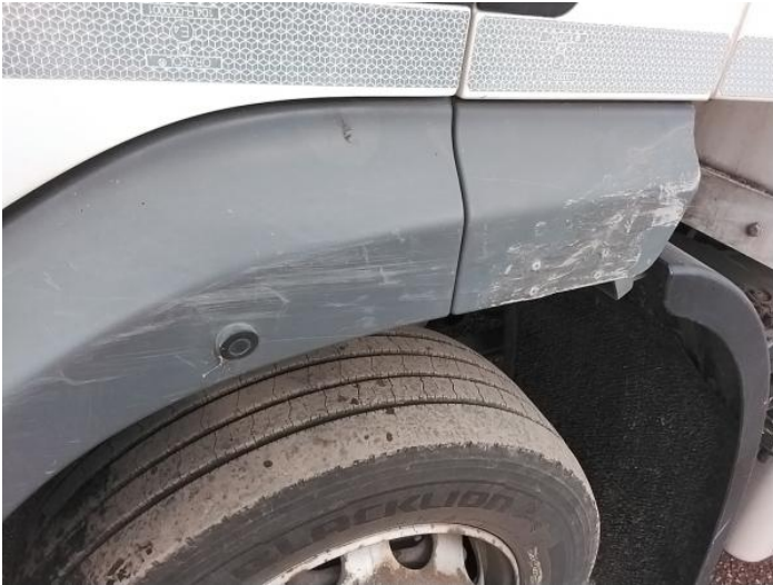
3: Wing nsf Poor Previous Repair Rippled Up To 30%
