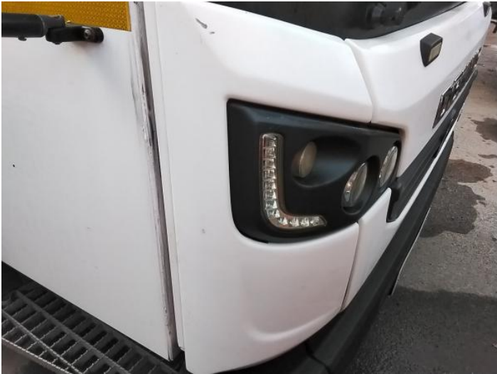
3: Panel Front Chipped Multiple Chips
