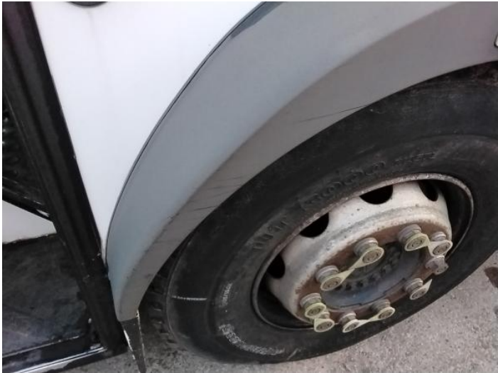
4: Wing nsf Scratched Over 25mm Thru Paint
