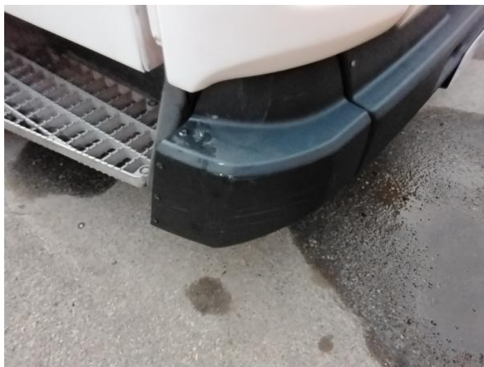
2: Bumper Front Scratched 25 to 100mm Thru Paint
