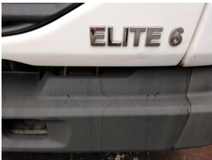
1: Bumper Front Grill Broken Replace
