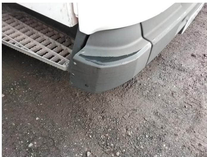
2: Bumper Front Scratched Over 100mm Thru Paint
