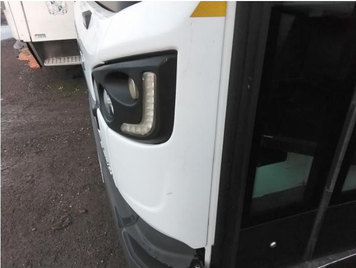
4: Panel Front Scratched Over 25mm Thru Paint
