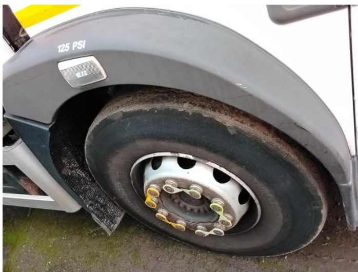
1: Wing osf Scratched Over 25mm Thru Paint
