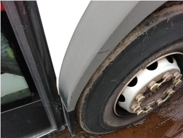
3: Wing nsf Scratched Over 25mm Thru Paint
