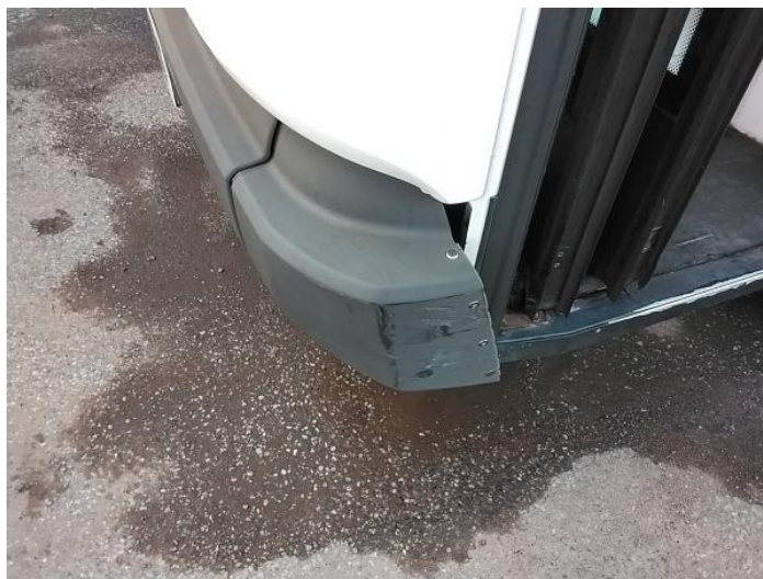
2: Bumper Front Scratched Over 100mm Thru Paint
