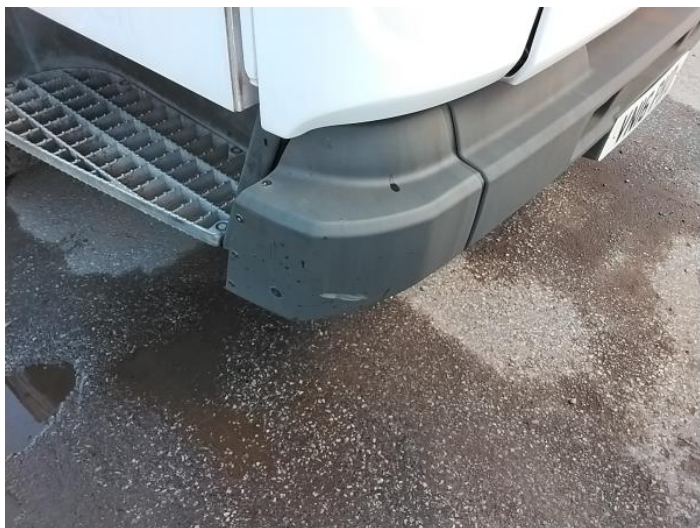
1: Bumper Front Scratched 25 to 100mm Thru Paint
