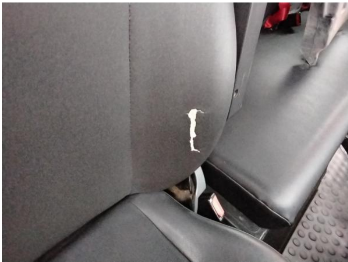
3: Seat Back Cover osf Torn Over 3mm
