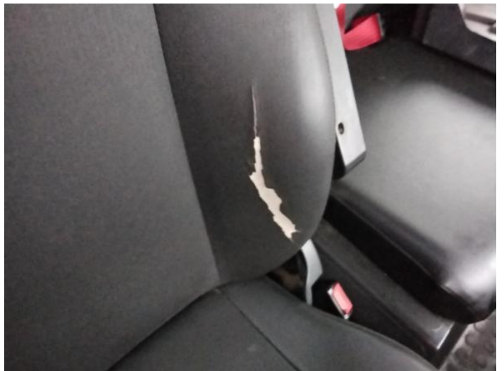
2: Seat Back Cover osf Torn Over 3mm
