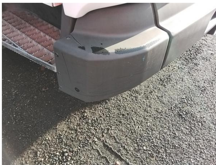
2: Bumper Front Scratched Over 100mm Thru Paint
