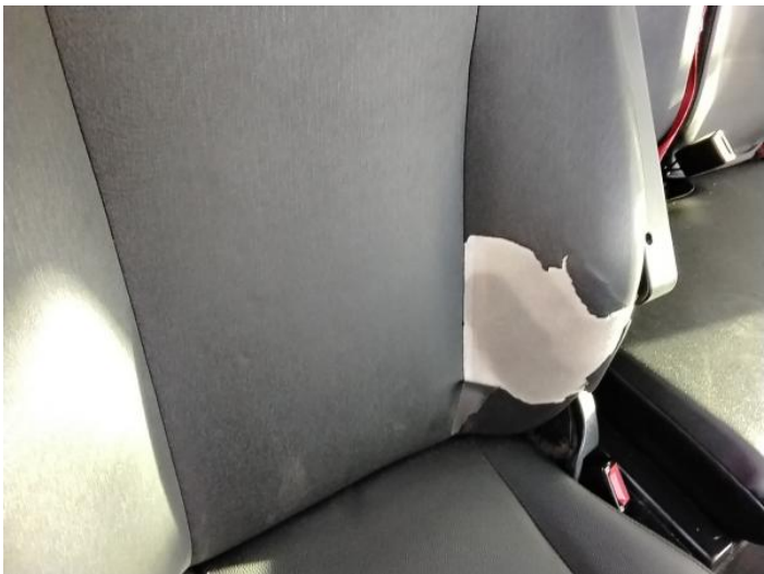
4: Seat Back Cover osf Torn Over 3mm
