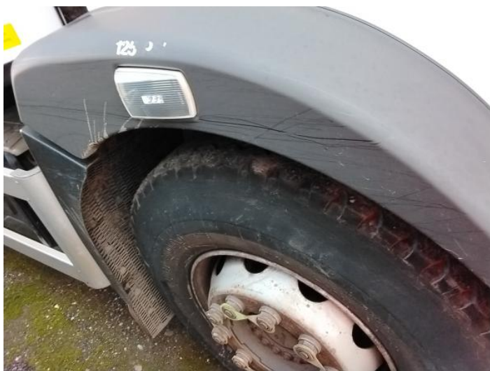
1: Wing of Scratched Over 25mm Thru Paint
