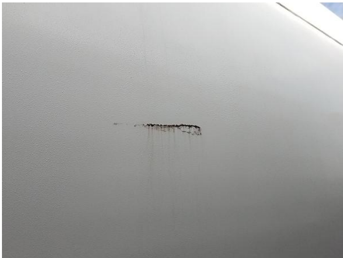
3: Qtr Panel nsr Scratched Over 25mm Thru Paint
