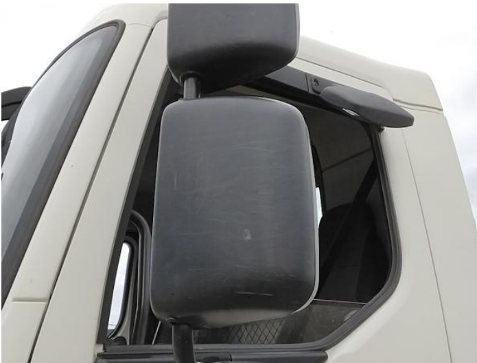
3: Door Mirror Assy nsf Scuffed (Unpainted) UpTo 100mm
