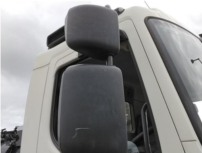
11: Door Mirror Assy osf Scuffed (Unpainted) UpTo 100mm
