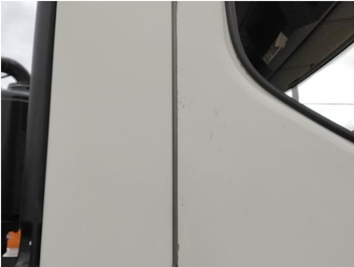
9: Door osf Chipped Edge Chip
