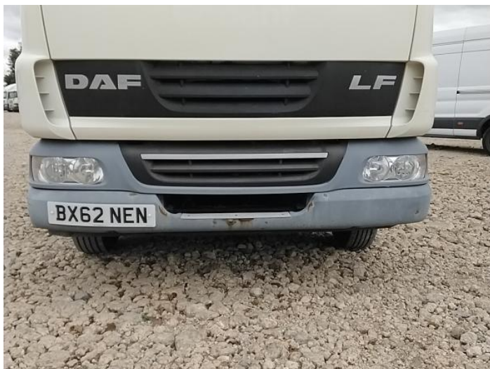
1: Bumper Front Rusted Over 5mm
