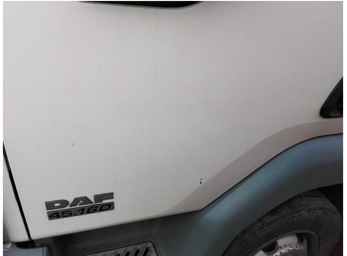
4: Door nsf Chipped Multiple Chips
