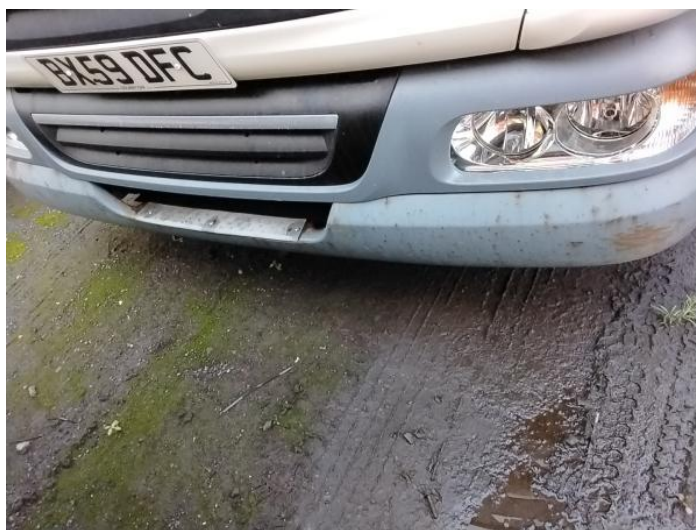
2: Bumper Front Rusted Over 5mm
