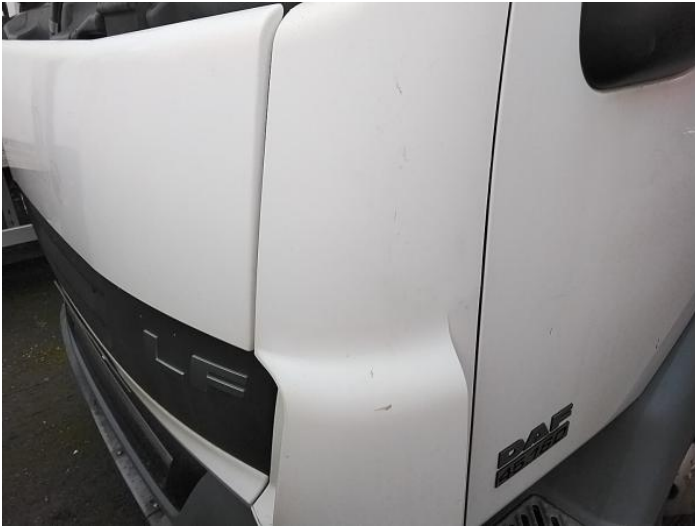
3: Panel Front Scratched Over 25mm Thru Paint
