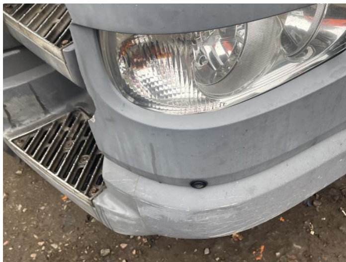
2: Bumper Front Moulding Broken Replace
