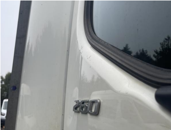
3: Door osf Dented Over 30mm
