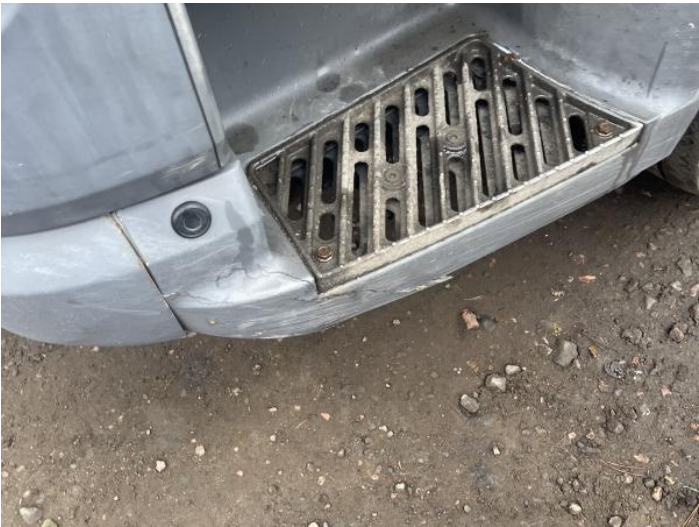
6: Door Moulding nsf Broken Replace
