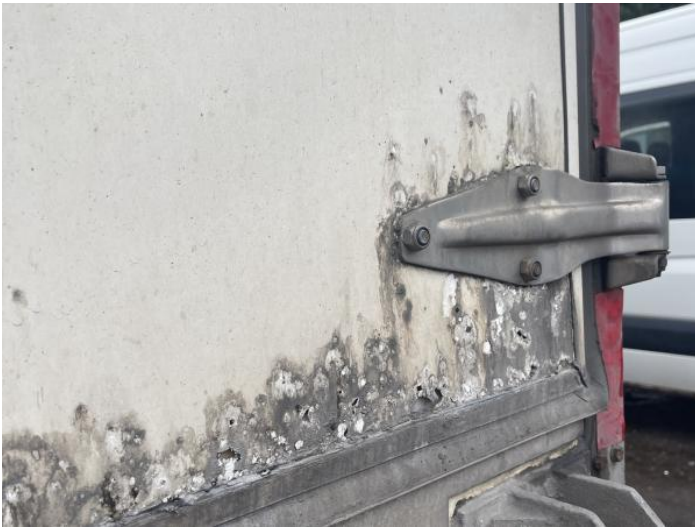
5: Tailgate Rusted Over 5mm
