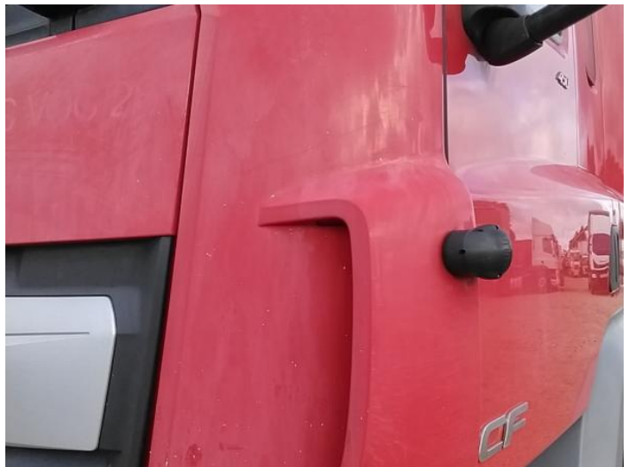
6: Wing nsf Cracked Replace
