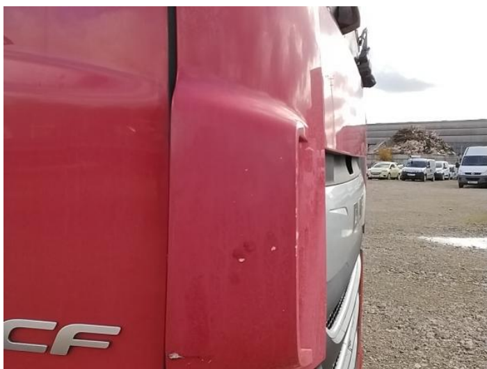
1: Wing osf Scratched Over 25mm Thru Paint
