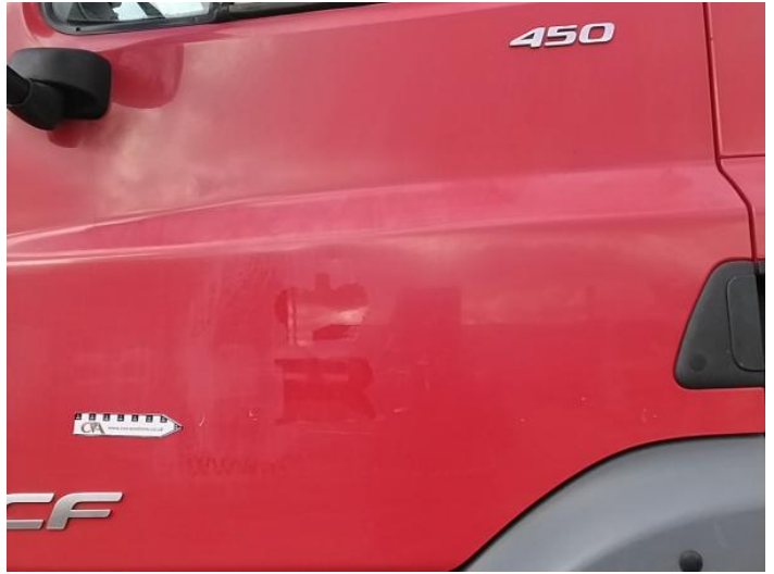
10: Door nsf Scratched UpTo 25mm Thru Paint
