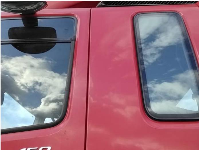
11: B Post ns Scratched Over 25mm Not Thru Paint
