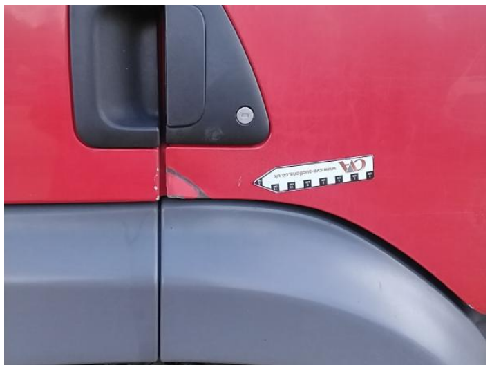
14: Door osf Dented With Paint Damage
