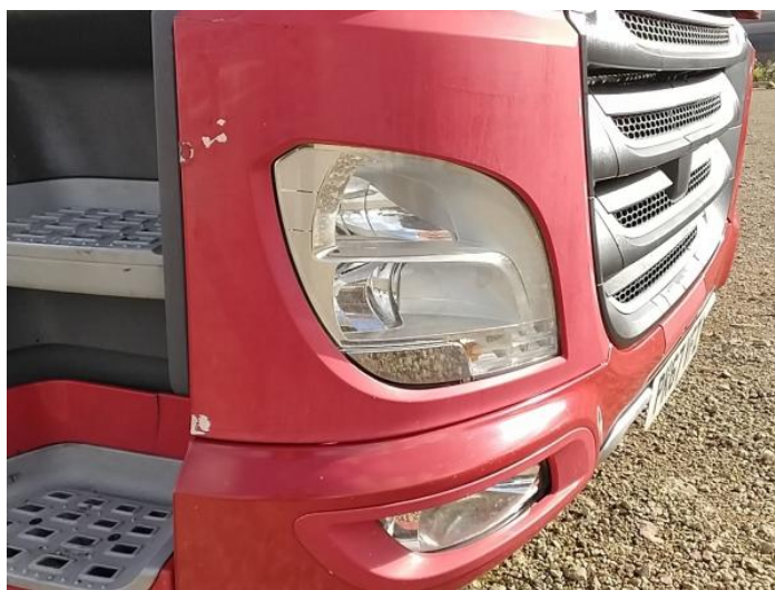
2: Fog Lamp Surround os Broken Replace
