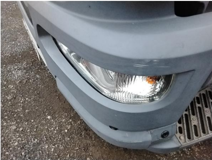
5: Panel Front Scratched Over 25mm Thru Paint
