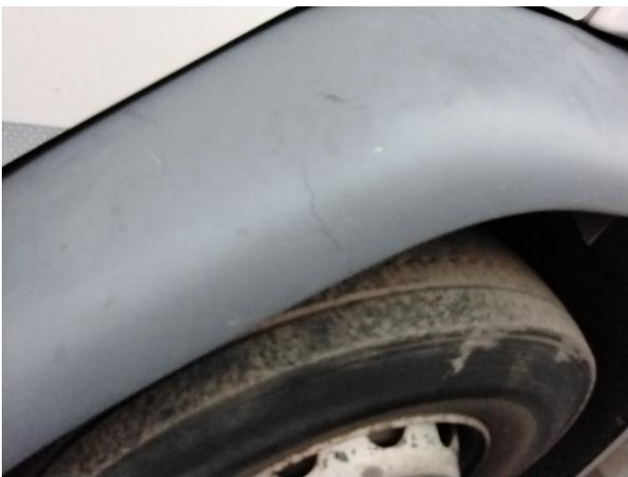
7: Wing nsf Cracked Replace
