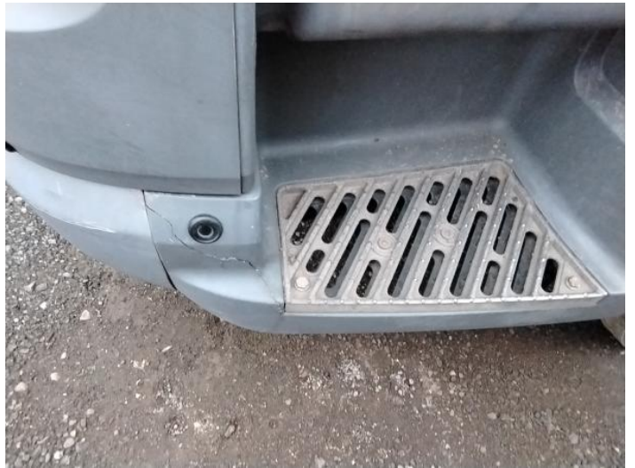
6: Bumper Front Moulding Broken Replace
