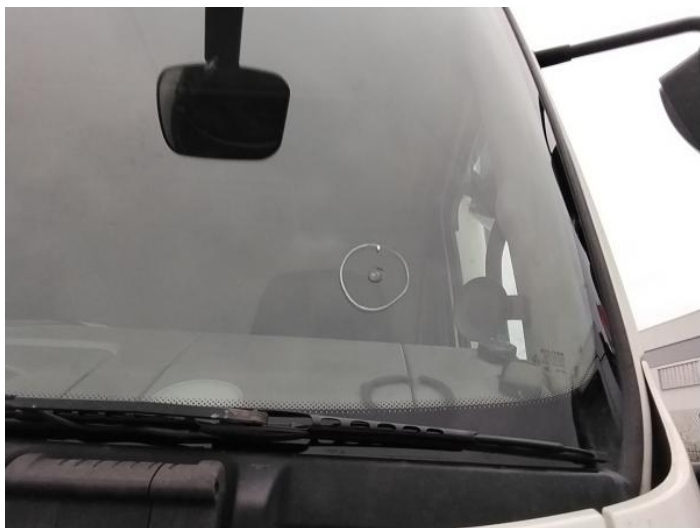
1: Screen Front Chipped Over 10mm
