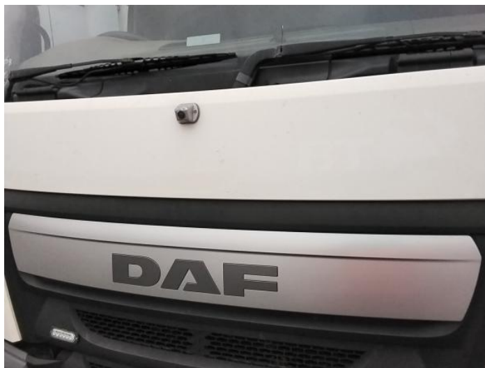
2: Bonnet Chipped Multiple Chips
