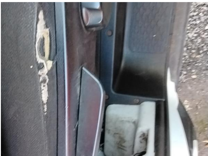
4: Seat Base Cover osf Torn Over 3mm
