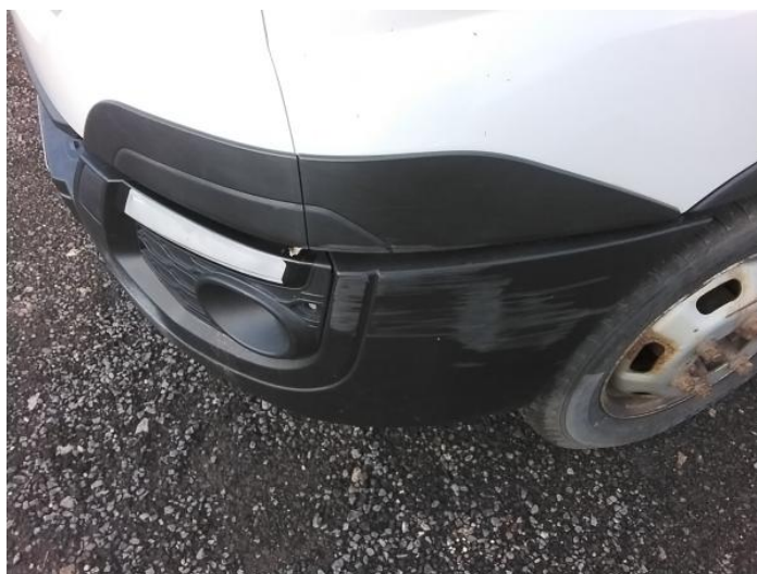
2: Bumper Front Scratched Over 100mm Thru Paint
