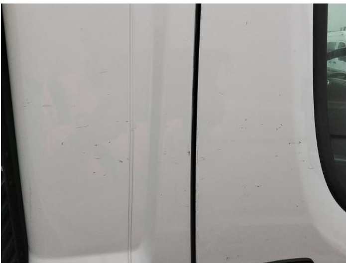
7: Door osf Chipped Multiple Chips
