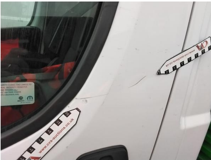
5: Door nsf Dented With Paint Damage
