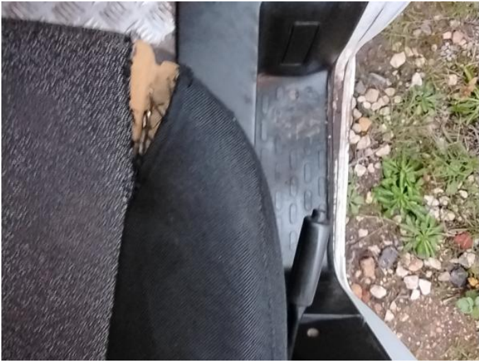
9: Seat Base Cover osf Torn Over 3mm
