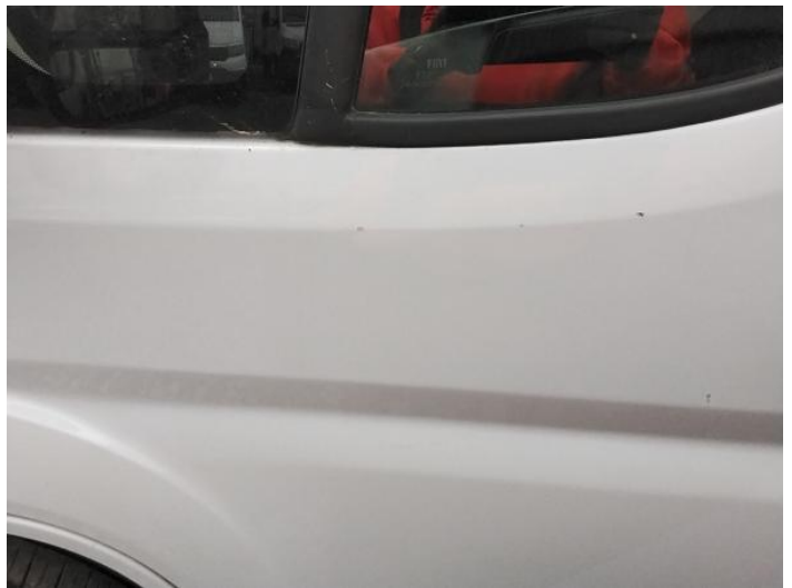
6: Door nsf Chipped Multiple Chips
