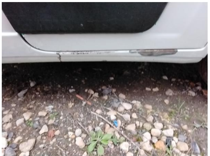
8: Sill os Scratched Over 25mm Thru Paint
