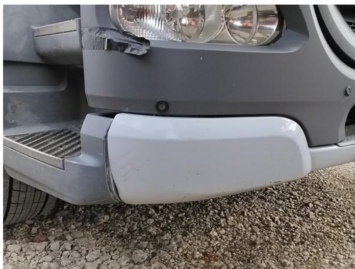
2: Bumper Front Moulding Scratched (Painted) UpTo 25mm Not Thru Paint
