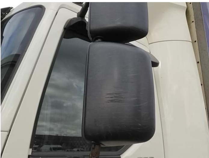
7: Door Mirror Assy nsf Scuffed (Unpainted) UpTo 100mm
