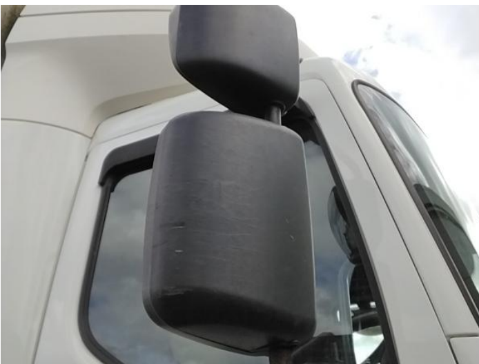
13: Door Mirror Assy osf Scuffed (Unpainted) UpTo 100mm
