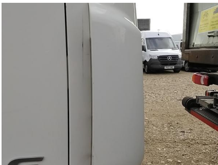
1: Wing osf Scratched UpTo 25mm Thru Paint
