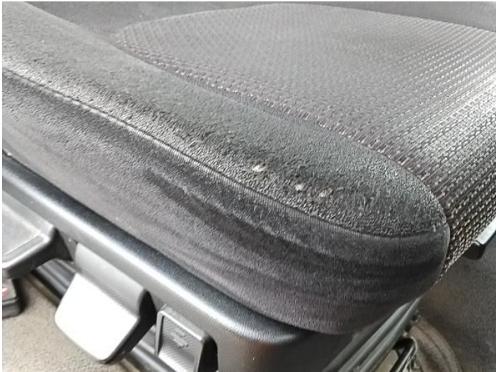
16: Seat Base Cover osf Holed Over 3mm
