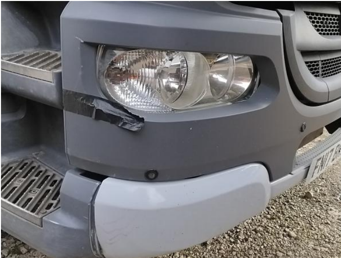
3: Fog Lamp Surround os Broken Replace
