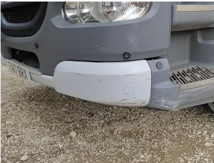
5: Bumper Front Moulding Scratched (Painted) Over 25mm Thru Paint
