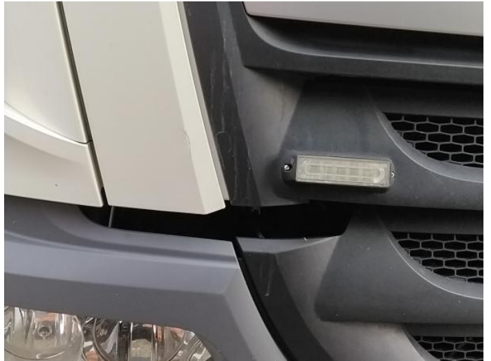
4: Bonnet Cracked Replace
