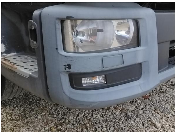
1: Fog Lamp Surrounds Scuffed (Unpainted) Up To 100mm
