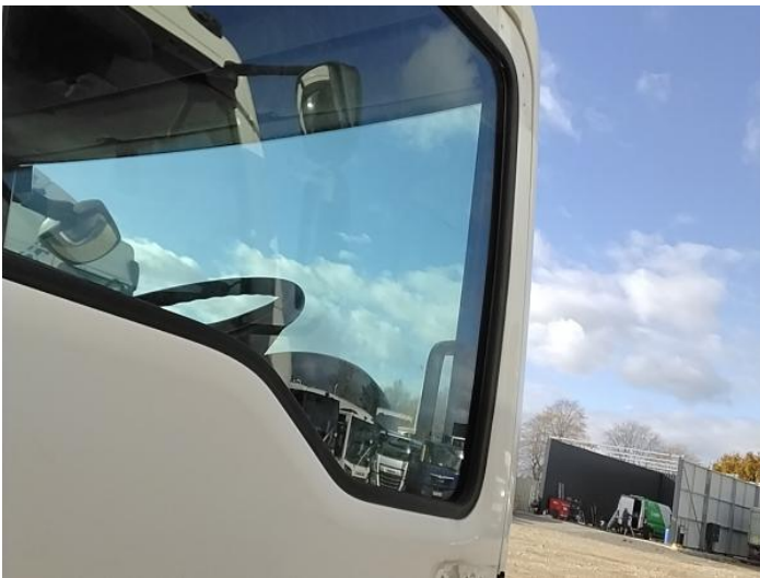
11: Door Mirror Assy osf Missing Replace
