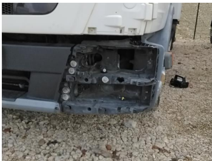
2: Headlamps Missing Replace
