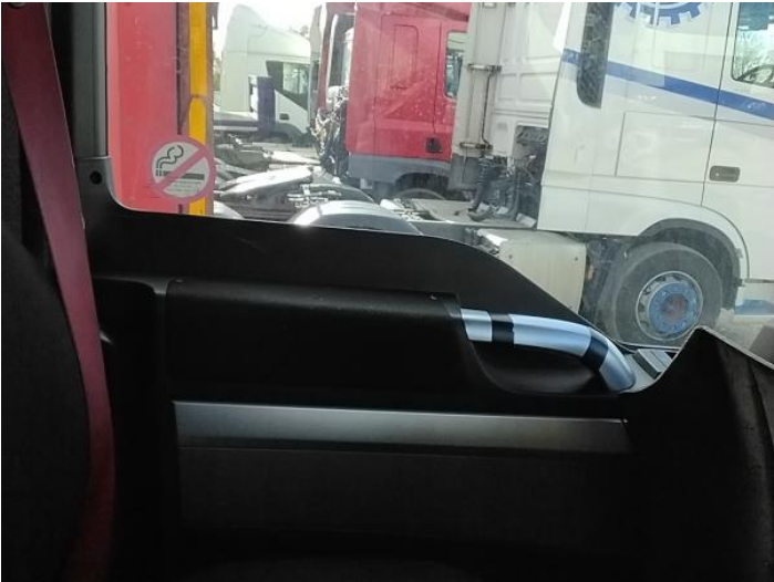
16: Handle Inner nsf Damaged Replace
