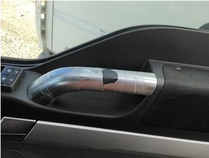
15: Handle Inner osf Damaged Replace
