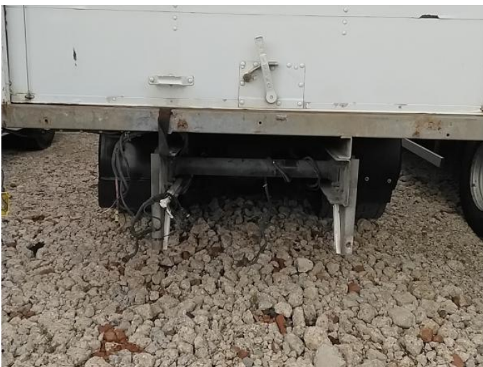
7: Bumper Rear Missing Replace
