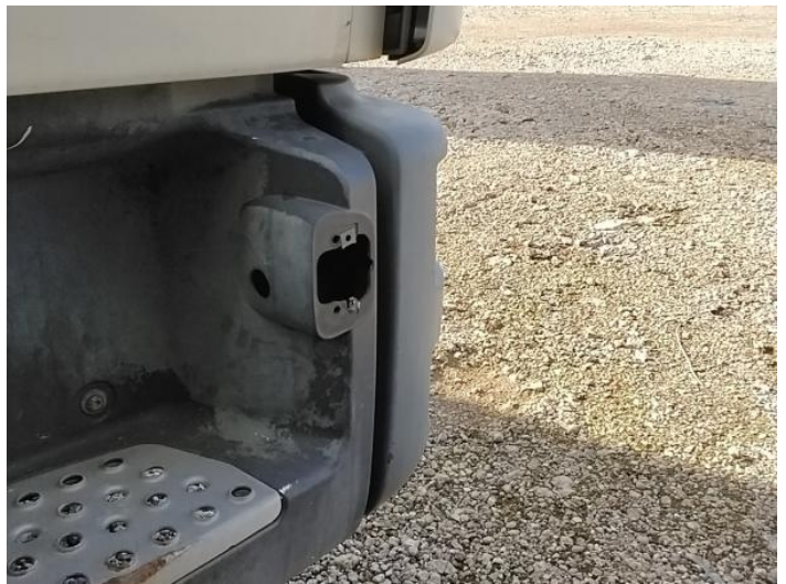
12: Flasher Side Repeater os Missing Replace
