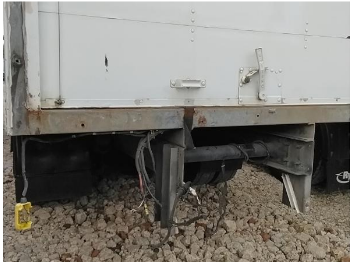
6: Lamp nsr Missing Replace
