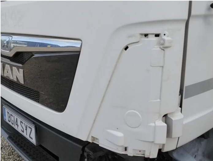
3: Wing nsf Missing Replace
