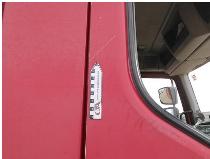
10: Door osf Scratched Over 25mm Thru Paint
