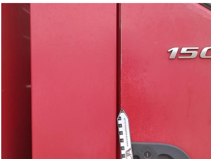
11: Door osf Chipped Edge Chip
