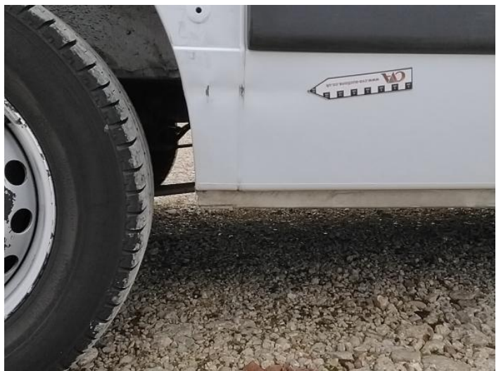
20: Qtr Panel osr Dented With Paint Damage
