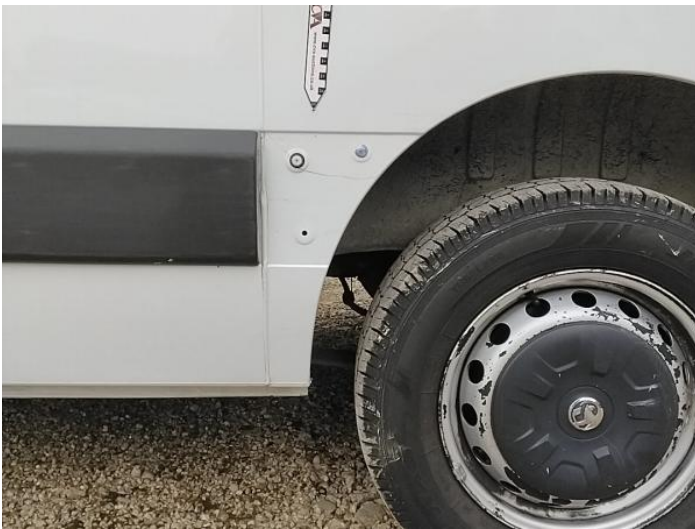
11: Qtr Panel Moulding ns Missing Replace
