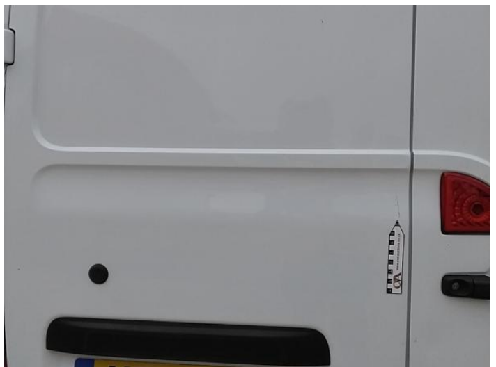
14: Door nsr Scratched UpTo 25mm Thru Paint
