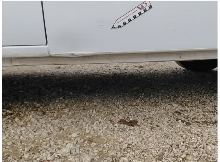
10: Sill ns Dented Between 10mm + 30mm
