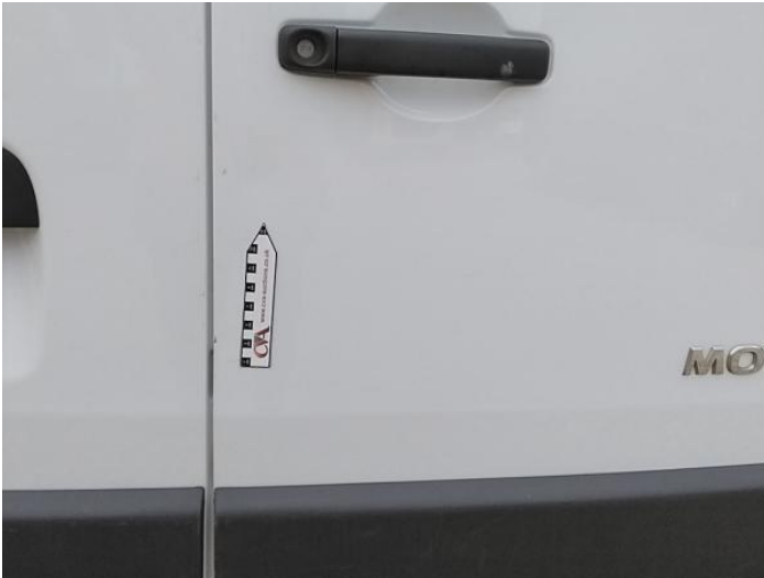
15: Door osr Dented Between 10mm + 30mm
