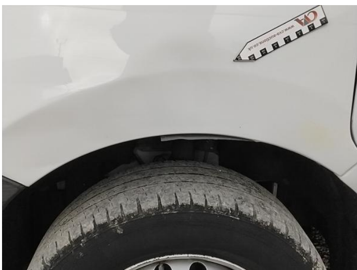
5: Wing nsf Dented Between 10mm + 30mm
