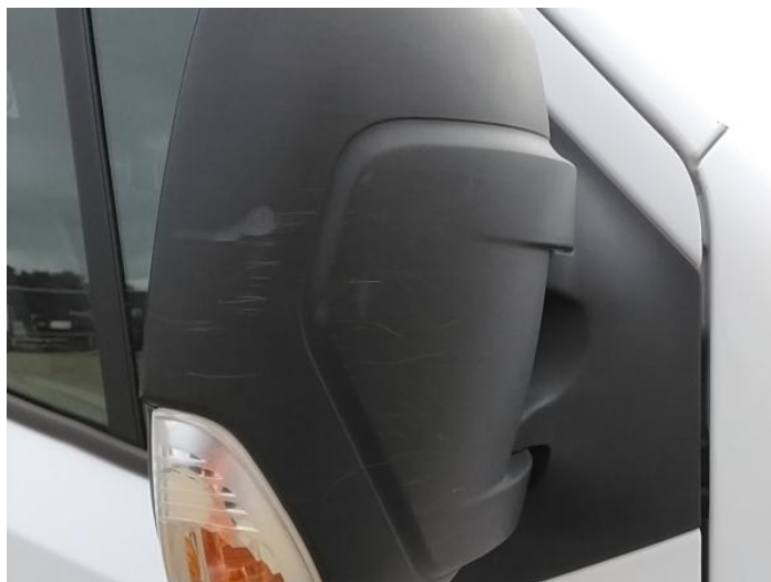
22: Door Mirror Assy osf Scuffed (Unpainted) UpTo 100mm
