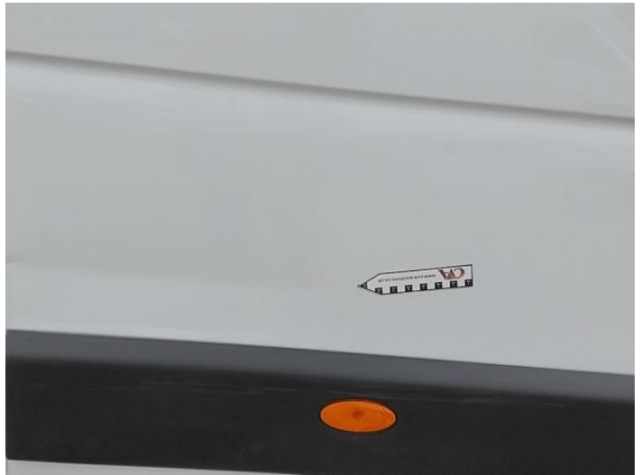
18: Qtr Panel osr Dented Between 10mm + 30mm
