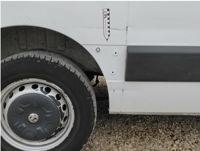
17: Qtr Panel Moulding os Missing Replace
