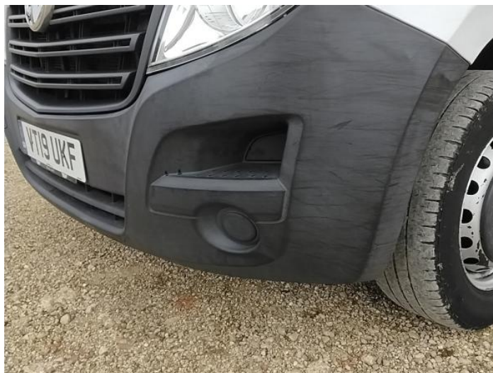
4: Bumper Front Moulding Scuffed (Unpainted) UpTo 100mm
