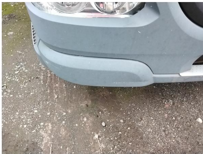
2: Bumper Front Dented With Paint Damage
