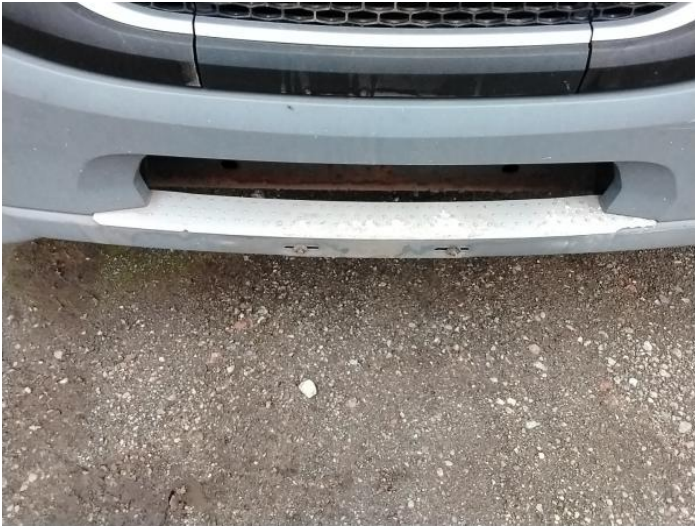
3: Number Plate Front Missing Replace
