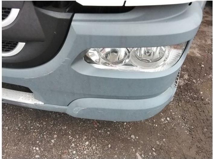
4: Bumper Front Scratched Over 100mm Thru Paint
