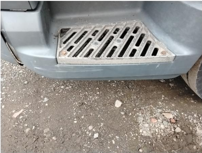
5: Bumper Front Moulding Scuffed (Unpainted) Over 100mm
