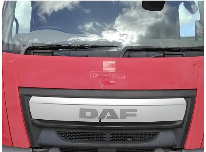
4: Bonnet Cracked Replace
