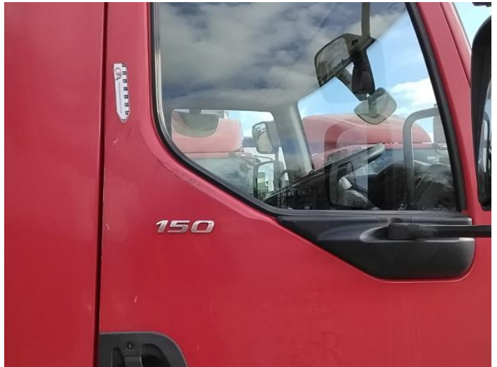
12: Door osf Scratched UpTo 25mm Thru Paint
