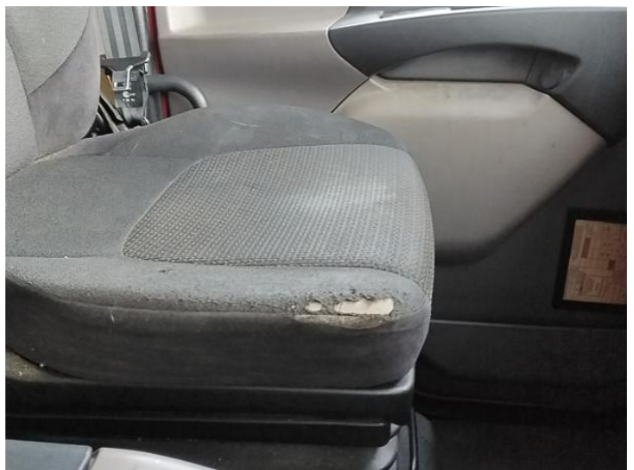
14: Seat Base Cover nsf Holed Over 3mm
