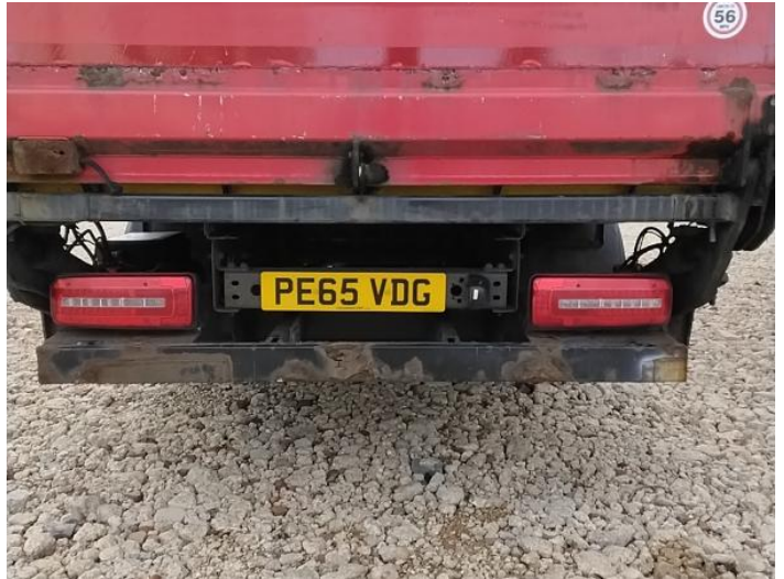
10: Bumper Rear Rusted Over 5mm
