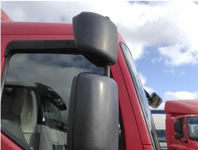
11: Door Mirror Assy osf Broken Replace
