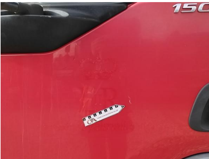
7: Door nsf Scratched UpTo 25mm Thru Paint
