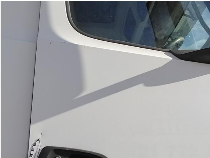
11: Door osf Scratched UpTo 25mm Thru Paint
