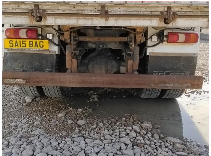
6: Bumper Rear Rusted Over 5mm
