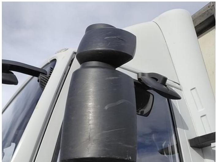
6: Door Mirror Assy nsf Broken Replace
