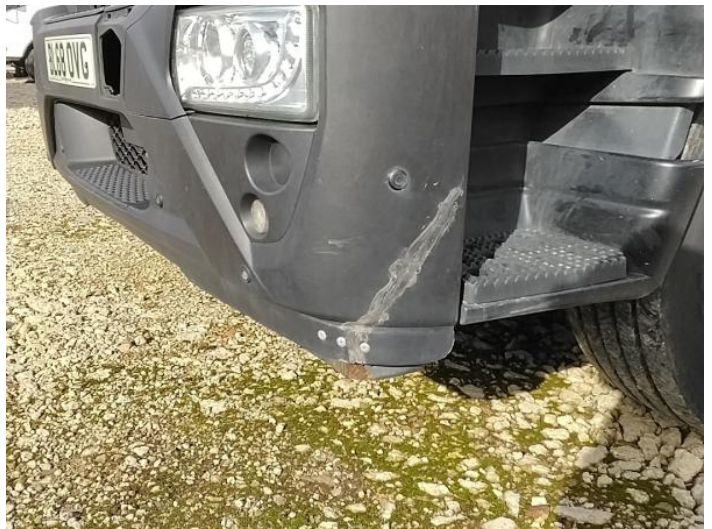
4: Bumper Front Moulding Broken Replace
