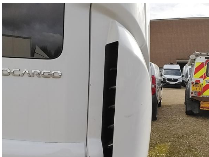
1: Wing osf Scratched Over 25mm Thru Paint
