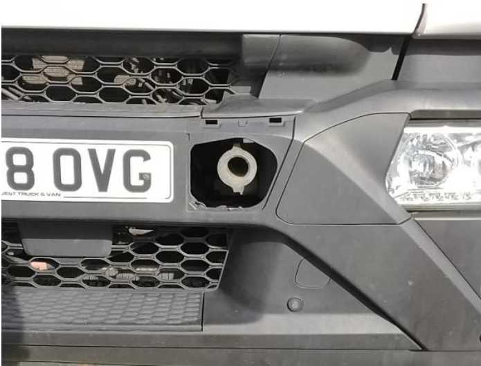
3: Front TowEye Cvr Missing Replace
