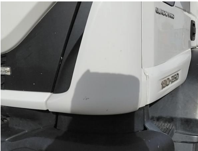
5: Wing nsf Scratched UpTo 25mm Thru Paint
