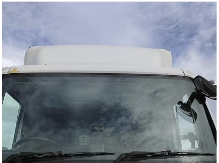
4: Screen Front Chipped UpTo 10mm
