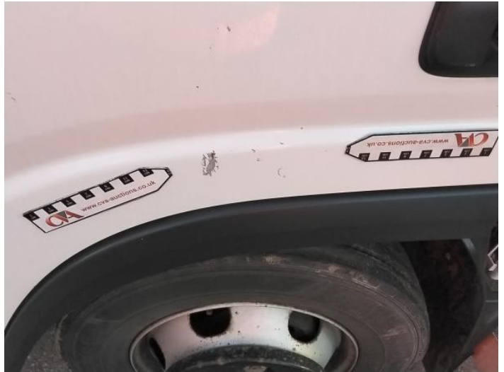
4: Door nsf Scratched Over 25mm Thru Paint
