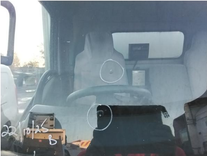
3: Screen Front Chipped Over 10mm
